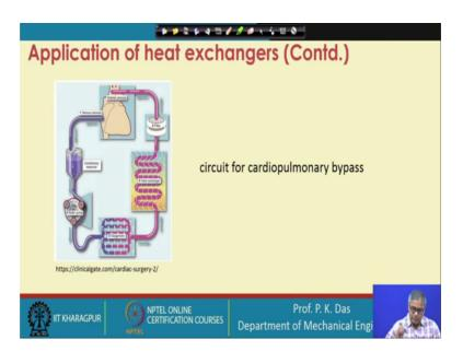
Just one example I have shown here, this is the circuit for cardiopulmonary bypass surgery and you can see that there are different component, but there is one heat exchanger, there is one heat exchanger, there is one heat exchanger over here and actually the blood is to be heated or cooled depending on because this is how the body temperature of the patient that can be also control and that is why we need a very good heat exchanger; these are unique kind of heat exchanger which are used.
