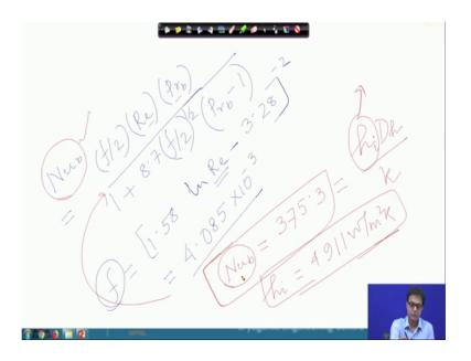
And as we have said that we will be using the Nusselt number at the bulk temperature as I have shown it, this is f by 2 into R e to the power this is P r that bulk divided by 1 plus 8.7 into f by 2 whole to the power half. And P r b minus evaluated at the bulk mean temperature divided minus 1.
