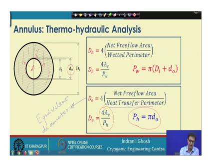
This equivalent diameter, now what is the heat transfer parameter? The heat transfer parameter, the heat transfer is occurring in terms of only through this area because we have the inner fluid flowing through this tube and the fluid flowing at the annular space another fluid. So, the heat transfer is taking place through this surface and that is related to pi d 0.
