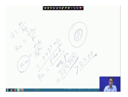
And then we can apply this relation G D h by mu to calculate the Reynolds number or we can also try to find out the velocity by m dot by rho AC. So, here if it is for the hot fluid it will be rho h AC, and you can find out it to be say 0.673 meter per second.
