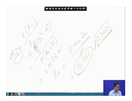
The hydraulic diameter can be calculated as how is the hydraulic diameter 4 times that free flow area, does just now we have calculated and that P w which is nothing but pi d 0 plus D i. And we have 4 times 4 by pi D square D i square minus d 0 square by 4, this is pi.
