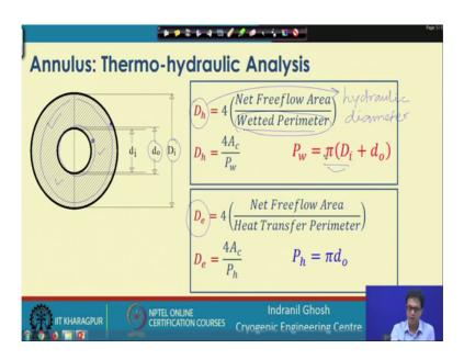
Whereas, the other part is the annular part; where in the annular part we have this heat transfer coefficient if we want to look for, or the heat transfer coefficient and the pressure drop, we have basically same correlation, but evaluated in terms of a different hydraulic diameter. Or equivalent diameter often we call this is the equivalent diameter this is the hydraulic diameter.
