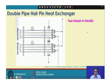
So, in parallel mode what happens? One of the fluid stream will be divided into 2 parts say for example. So, one of the fridge stream is coming over here it is divided into 2 part, one part is entering to this fluid stream and it will carry on like this. The other part will be distributed to the second hairpin. So, this is entering here this is entering at this point.
