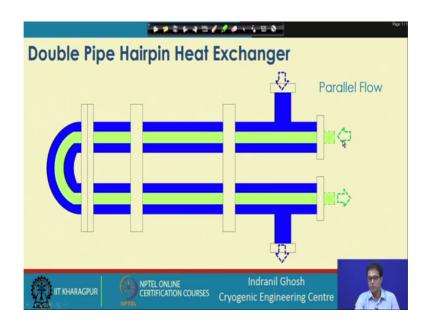
Now looking into the construction of this geometry, we see that these 2 are the support structures to keep it in position whereas, these are generally flanged connection. So, if we remove this part, we are able to clean this heat exchanger easily. So, that keeps a pretty good advantage for this type of exchangers that, we can clean it easily and we can use it for dirty environment or the fluids handling dirts can also be used for this in this exchanger.
