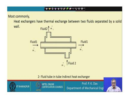
Most commonly heat exchanger have thermal exchange between 2 fluids, though we have given a general description of heat exchanger definition of heat exchanger that it can be heat exchanged between number of fluids or there could be heat exchange between a fluid and the solid. But most of the heat exchanger will have only 2 fluids and probably we are having probably we are having the most basic most basic construction
