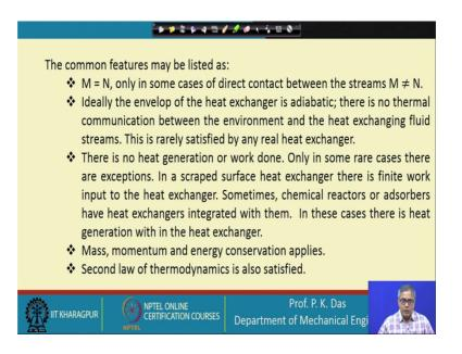
But there can be some exception M is equal to N only in some cases of direct contact M is equal to N in most of the cases only in some cases of direct contact between these streams M is not equal to N, otherwise heat exchangers are indirect contact and M is equal to N. Ideally the envelope of the heat exchanger should be insulated, but in most of the cases it is not in practical heat exchanger real heat exchanger it is not.
