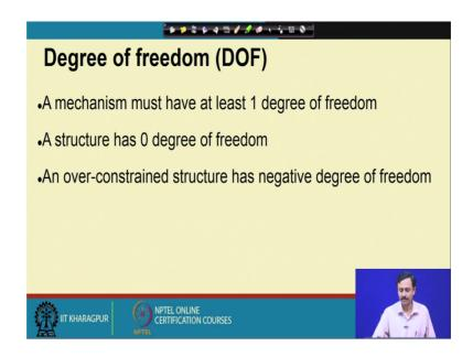
Then we also discussed that a mechanism must have at least 1 degree of freedom. A structure has 0 degree of freedom and an over-constrained structure has negative degrees of freedom.
