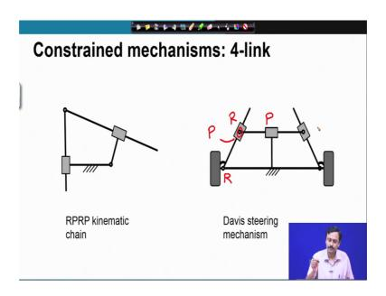
Then RPRP kinematic chain, this is the Davis steering mechanism which use the RPRP kinematic chain, but there are two copies of this kinematic chain; let us mark them out. So, this is R; here you have a P, this is the next R and this is the P and then there is another set of RPRP for the other wheel. So, this is the Davis steering mechanism; which uses the RPRP kinematic chain.
