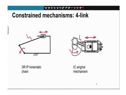
So, these are applications of the 4R kinematic chain; 3R1P, a very standard application is an ice engines. So, you have this piston which is oscillating; so, this is our PPR and this is connected to the crankshaft and this is the coupler; this is the connecting rod.
