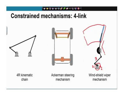
Let us now look at some applications say 4R kinematic chain; we have looked at this Ackerman steering wheel mechanism; we also have this windshield wiper mechanism. So, here is the wiper which is going to wipe the windshield or windscreen. So, here you have a motor which is rotating this link; this is the coupler and so 3, 2, 1; 1 is the ground, 2 is the crank here. So, this link; 3 is the coupler and 4 is connected to the wiper.
