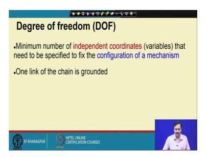
So, just to review what we have discussed previously; so, degree of freedom is a minimum number of independent coordinates that need to be specified to fix the configuration of a mechanism; one link of the chain is grounded.
