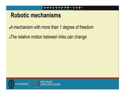
Now, in this course we will define robotic mechanisms as those which have more than 1 degree of freedom; that means, two or higher; they will be termed as robotic mechanisms. Now as I have told you in mechanisms with degree of freedom more than 1; that means, 2 or higher; the relative motion between the links can change. Now that is an advantage and in some situations or in a way that brings in some complicacy; so that is what we are going to look at now.
