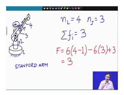
Then we have this robotic mechanism; this is known as the Stanford Arm; let us calculate the degree of freedom of this. Now this is a spatial mechanism as you can see; let me fix this as ground, with respect to this ground, this cylindrical member can rotate as has been shown. So, ground is 1; this cylindrical member is 2; this is 3 and the slider is 4.
