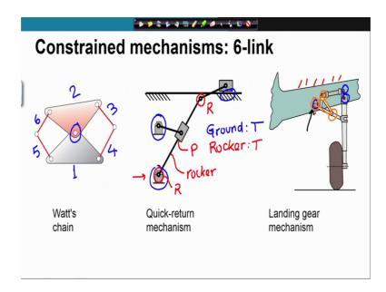
Let us go over to 6-link where we have been talking about 4-link kinematic chain, now we go to 6-link kinematic chain this is called the Watt's chain. So, it has got two ternary links as you can see; so 1, 2, 3, 4, 5, 6, so links 1 and 2 are two ternary links and these two ternary links are connected at this kinematic pair.
