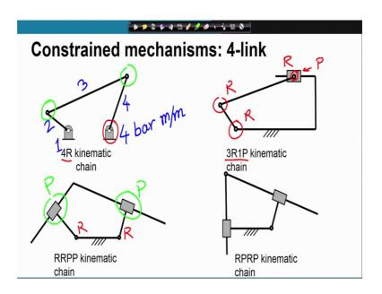
Let us look at some examples of constraint mechanisms. So, this is a four link constraint mechanism; we have seen this. So, ground is 1, this is 2, this is 3, this 4, so we call it a 4 link mechanism or if sometimes a 4 bar mechanism.
