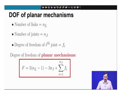
And we have looked at this calculation in detail. So, this is for the planar mechanism; where I would like to point out that here for a planar mechanism, we have 3 because in a plane every rigid body has 3 degrees of freedom.
