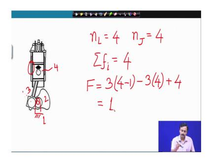
This is an ice engine remember that this is the crankshaft.
