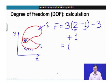
Now, we look at this example, we have two links now connected by a kinematic pair. So, this forms a chain as we had discussed, I will ground one body. If I ground one body immediately it loses all its degrees of freedom. So, right now I have this rigid body this link which can move. So, without this kinematic pair, let us see without this kinematic pair this body has 3 degrees of freedom. This body had 3 degrees of freedom, but I have grounded it.
