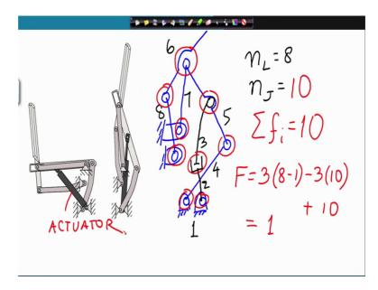
Let us move over to this transfer device, let me draw the kinematic diagram first, here you can see there are two ground hinges. Here there is a an actuator, here there are two more ground hinges this one is connected like this, and from here it is connected like that. So, this is the kinematic diagram. So, let me count the number of links. So, ground is 1 2 3 is the two links which have the prismatic pair, 4 the ternary link has 5 6 7 and 8.
