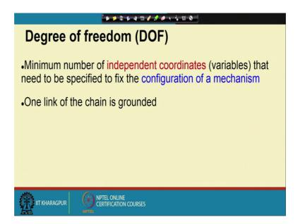
So, here I have written out the formal definition, is the minimum number of independent coordinates or variables that need to be specified to fix the configuration of a mechanism. So, minimum number of independent coordinates, and configuration of mechanism these are the keywords.
