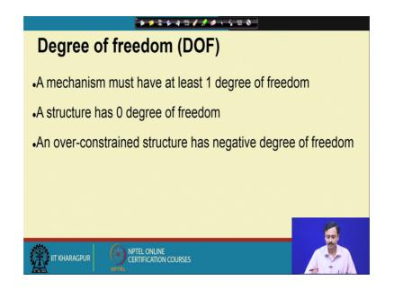
Now, let us see what a mechanism must be in terms of its degrees of freedom. As I have mentioned right at the outset that a mechanism is something that can move. So, it must be able to move, it must have at least 1 degree of freedom. So, from this calculation we can now determine the degree of freedom of a combination or an assortment of links connected by certain kinematic pairs. Now if this assortment or this combination has to move then it must have at least one degree of freedom.
