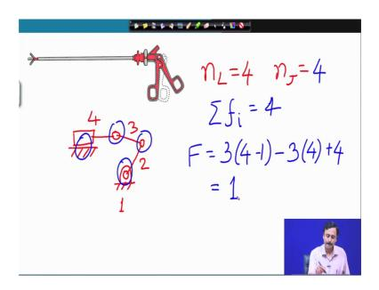
This is the surgeon's tool. First I will quickly draw the kinematic diagram as we have seen.
