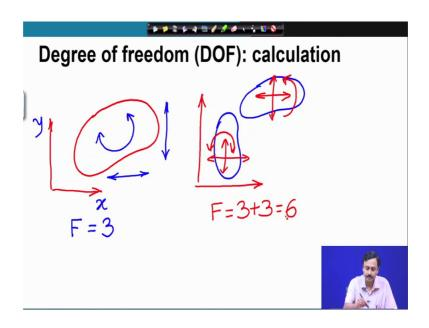
Let me start with a simple thing a planar body. So, a body on a plane; as you know this link this body has 3 degrees of freedom, what are the 3 degrees of freedom? It can move along this coordinate let me call that as x, it can move along y and it can rotate in the plane.
