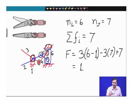
Let us look at this scissors, again I need to draw the kinematic diagram. So, this was the kinematic diagram this is a ground hinge. So, ground is 1 2 3 4 5 6 is the slider.
