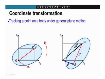
Now, let us go to the general plane motion. So, a general plane motion; a body can not only rotate, but it can also translate. Here I have shown you a body which is not only rotating, but also translating. The point which was at the origin of the frame here I have this point P on the body and I have a point let us say Q sitting at the origin. Now this point Q has moved to this point under this general motion and P has moved here; our objective is to determine this vector p in frame 0.
