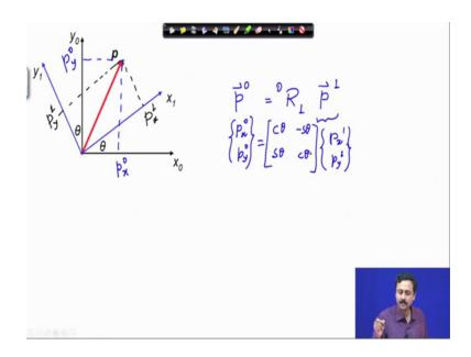
So, we have looked at the construction of the rotation matrix, which relates the body fixed coordinates  $p \ge 1 p \ge 1$ . So, from  $p \ge 1 p \ge 1$  we can obtain  $p \ge 0 p \ge 0$ .
