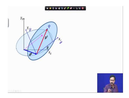
Under general motion the body moves like this and the frame also moves in this manner. So, I have the frame x 1 y 1 here which is fixed with the body and the point p is currently here. (Refer Slide Time: 14:07)
