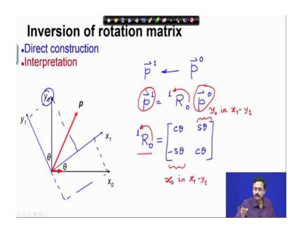
Now, the inverse rotation matrix which is to say that I have the representation of p in frame 0, I would like to take it. So, I have the representation in frame 0, I want to take it to frame 1, I want to represent the same vector p in frame 1. So, which means I will write the rotation matrix as from 0 to 1, p in frame 0 this rotation matrix R 0 to 1.
