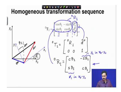
Now, if you have a sequence of rotations I have first x 1 y 1. So, a body moves from x 0 y 1 0 to x 1 y 1 and this x 1, y 1 to x 2, y 2 in the frame x 2 y 2 we have the vector p 2, I would like to find out relation between p 0 which is in frame x 0 y 1 0 and p two which is in x 2 y 2.
