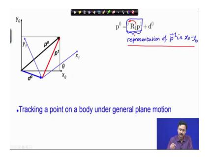
Through the rotation matrix I have brought p 1 in frame 0, through the rotation matrix R 1 to 0, I have found the representation of p 1 which is in x 1 y 1 as a vector in x 0 y 0.
