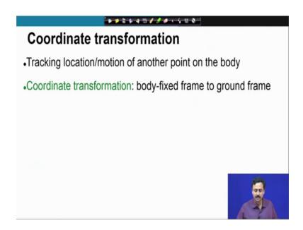
A coordinate transformation helps us in tracking or locating points on a body, which is in motion. So, our coordinate transformation will give us the coordinates of a point in a body, which is moving it will give us the coordinates of the point in the ground fixed frame; so, that is the purpose of coordinate transformation. So, it transforms from a local body fixed frame to a ground fixed frame.
