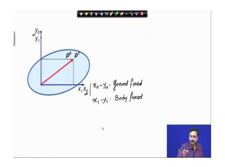
Here I have shown you the situation once again right from the beginning, I have a frame  $x \ 0 \ y \ 0$  which is fixed ground fixed and  $x \ 1 \ y \ 1$  is body fixed. So,  $x \ 0 \ y \ 0$  is ground fixed  $x \ 1 \ y \ 1$  is body fixed.
