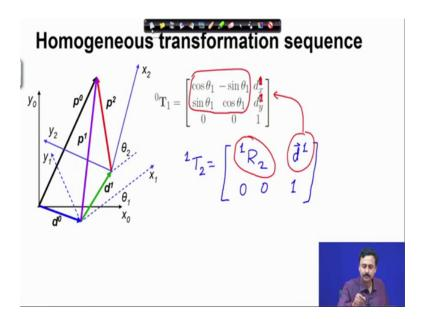
Now let us move to the second sequence the second motion, when it goes from x 1 y 1 to x 2 y 2, there is the same thing here the matrix the homogenous transformation matrix T from 2 to 1 is nothing, but R from 2 to 1 0 0 and here I have d represented in frame 1 and finally, here we have a 1.
