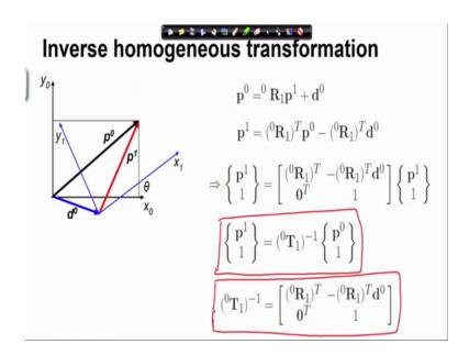
So, here I am formally showing you the steps this is what we finally, obtained this is our representation where the inverse homogeneous transformation matrix is given here.
