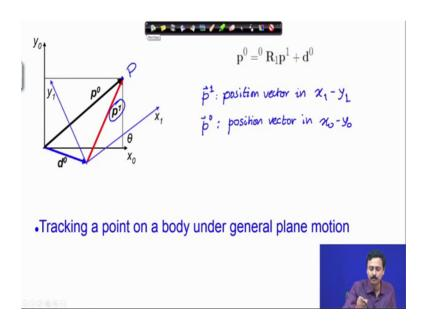
So, our objective is to determine the position vector p naught in frame x 0 y 0 of the point p. So, this is our objective to represent p naught the position vector of p in x 0 y 0 under a general motion of the body. Here I have shown the process schematically, we are tracking this point p under general motion. In the body fixed frame the vector representation is p 1, p 1 is a representation of p in x 1 y 1.
