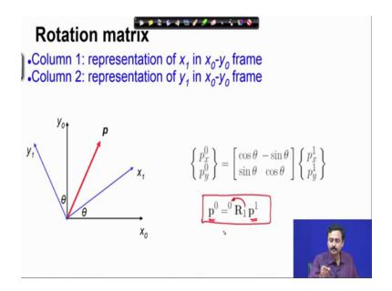
So, this is how we finally, represent the transformation. So, a vector in frame 1 is being taken to a vector in frame 0 and that is how we are representing the rotation matrix.
