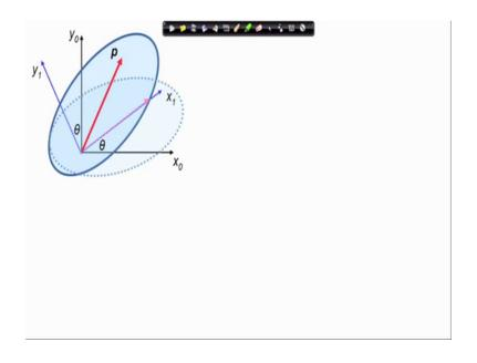
Here I have shown you x 0 y 1 0 as the ground fixed frame and x 1 y 1 as the body fixed frame as the body rotates; the body fixed frame also rotates with that and the point P takes up a new location.
