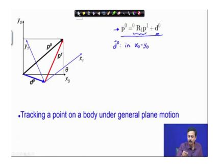
d 0 is represented in frame 0 d 0 has been represented in frame x 0 y 0.
