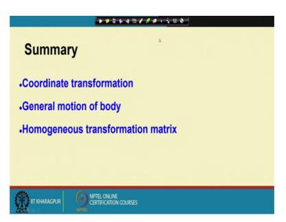
So, let me summarize we have looked at the coordinate transformation for a general motion of a body in plane in a plane, we have discussed the rotation matrix and the homogenous transformation matrix which is nothing, but a multiplicative factor, which you multiply with the extended position vector in the local frame to get the position vector in the world in the body in the global frame or the earth fixed frame.
