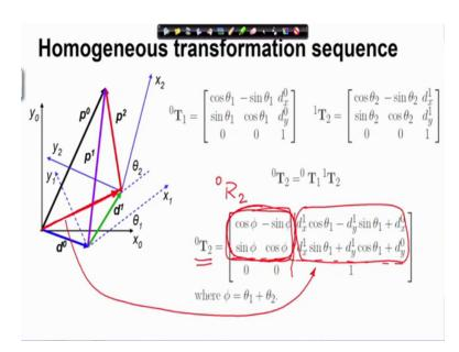
Now, if I want to find out the transformation from 2 to 0 then I just multiplied. So, transformation from 2 to 0 is transformation from1 to 0 times the transformation from 2
