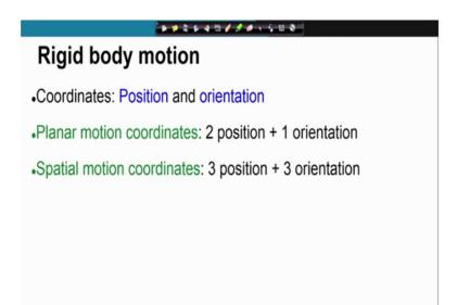
As we have discussed earlier, a rigid body motion requires position and orientational coordinates of the body to be tracked. For planar motion we require two position coordinates and one orientation coordinate whereas, in spatial coordinate a spatial motion of the rigid body we require three position coordinates and three orientation coordinates.
