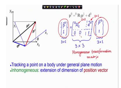
Now you see that this relation is inhomogeneous between  $p \ 1$  and  $p \ 0$  this is inhomogeneous. We have set out to relate  $p \ 1$  and  $p \ 0$ , but now we have a relation which is inhomogeneous, in homogeneity turns out to be because of this additional term d 0.
