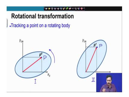
So, we have discussed this, we will review this once again the rotational transformation. So, we need to track the position of a point let us say P in a body as it rotates and comes to this configuration II from configuration I; So, the point p has moved to this new location, I would like to find out the coordinates of point p in the fixed frame x 0 y 1 0. So, that was the objective of the rotational transformation.
