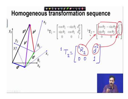
So, here I have the homogeneous transformation matrix T 2 1, which is R from 2 to 1 d 1 0 0 1. So, this R from 2 to 1 is this matrix and d 1 is this vector. So, that is the homogeneous transformation matrix 2 to 1.
