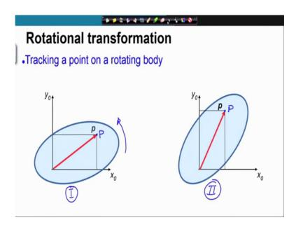
So now, we are going to directly go into the problem of tracking a point on a rotating body.
