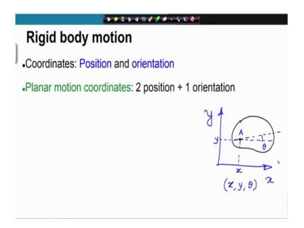
Now, rigid body motion is tracked by certain coordinates. So, how do you track a body moving in space a rigid body moving in space; or on the on the plane?
