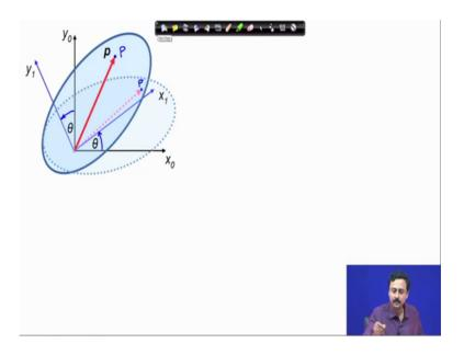
X 1 y 1 has rotated by this angle theta as you can see. This was the initial position of point P. And now, the new position of point P is here. Our objective is to locate the new point P in x 0 y 0. Here, I have removed the original position of the body in configuration 1. So, we can only see the body in configuration 2. The body fixes frame x 1 y 1 and the ground fixed frame x 0 y 0. We can also see the new location of point P.
