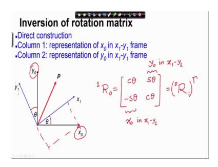
So, therefore, once again a direct construction let us look at it in direct construction of R from 0 to 1. So, what do I now have to do? I have to represent the frame x 0 y 0 in x 1 y 1. So, frame the axis x 0 the first column will be axis x 0 in x 1 y 1. So that, you can easily check is cosine theta this angle being theta. So, cosine theta and minus sin theta that represents x 0 in x 1 y 1.
