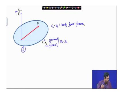
So, here, I have shown you a body in position 1 which rotates and goes over to position 2. There is a point P on the body, whose position vector is this vector p.
