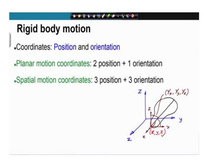
For spatial motions, we require 3 position coordinates and 3 orientations coordinates. Suppose, I have a body in which a line is fixed, then I can locate coordinates of a certain point on the body and the orientation by looking at possibly the direction cosines, these angles, that the line makes with the local xyz coordinate system, which is parallel to the blue coordinate system.
