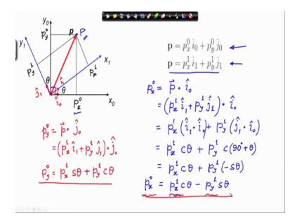
So, this is the new location of point P. What I want to determine is, this p x represented in frame 0 and p y represented in frame 0. In terms of p x represented in frame 1 and p y represented in frame 1.
