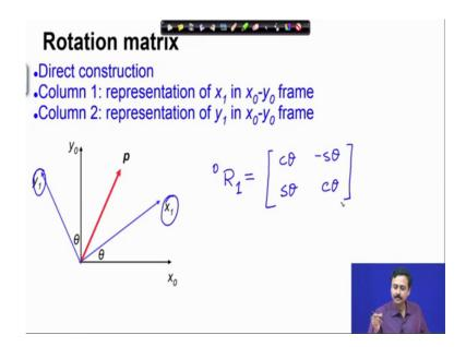
So, we can directly construct the rotation matrix. Let me do that. So, I say, that I want to construct this rotation matrix from 1 to 0 that will take me from frame 1 to frame 0, then I must represent the individual axis of the frame 1 in frame 0. So, frame 1 the first axis is  $x \cdot 1$ . So, let me represent  $x \cdot 1$  in  $x \cdot 0$  y 0.
