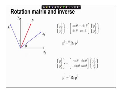
So, therefore, here I have written out the direct and the inverse rotation matrices from frame 0 to 1 and 1 to 0.
