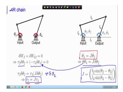
So, therefore, work done the virtual work done at the input plus the virtual work done at the output must sum up to 0 as for the principle of virtual work. Now, what is the virtual work done at the input the virtual work done at the input is torque at the input tau 2 times the virtual displacement at the input delta theta 2.
