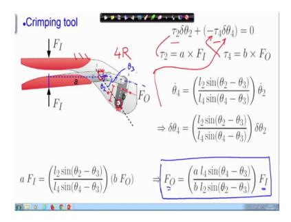
So, here I have this crimping tool and right at the beginning of this course. I had told you that this crimping tool can produce very high forces at the output. Here, I have denoted by FO the force at the output and FI the force at the input. Now, let us see the transformation of forces in this crimping tool.
