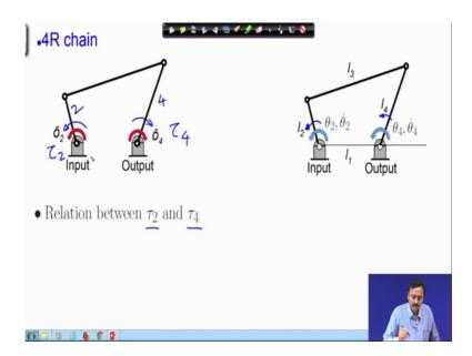
So, this shows the 4R chain I have shown the input torque. So, I have a torque T2 at the input and torque T4 at the output.
