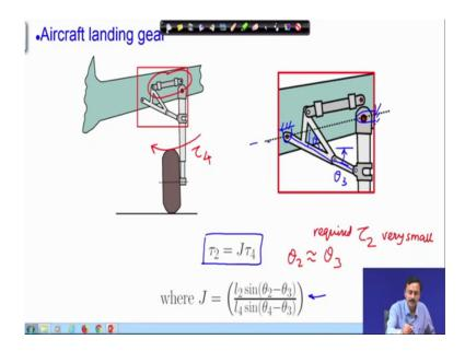
Similarly, in the aircraft landing gear, if you look at the mechanism in the aircraft landing gear, this is again a 4-bar mechanism. And here also, theta 2 this dashed line is the line of frame and this is theta 2 and this is theta 3.
