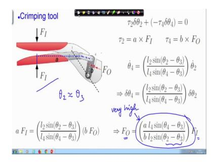
You can see that theta 2 and theta 3. So, link 2 and link 3 are almost collinear which means that theta 2 must be almost equal to theta 3. In that case, this denominator goes to 0 because theta 2 is almost equal to theta 3.
