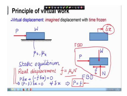
With this example, what I mean by virtual displacement? What I mean by time frozen? What I mean by force being frozen? So, here I take an example of a block of a certain weight on a rough surface with mu S, as the coefficient of static friction and mu K as a coefficient of kinetic friction. So, there is a rough surface on which we have a block of weight W and this is being pushed by a force P. Such that this system is in equilibrium it is in static equilibrium.
