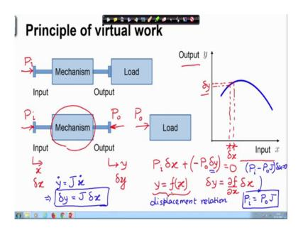
So, here again I explained the principle of virtual work for a mechanism that we are going to use. So, I have a mechanism at the input of which I have some input force. That is a P i and at the output it is driving certain load. So, this mechanism is given some input force and the load is driven by a certain force P o which is provided actually by the mechanism and on the mechanism therefore, by Newton's third law I must have P o in this direction.
