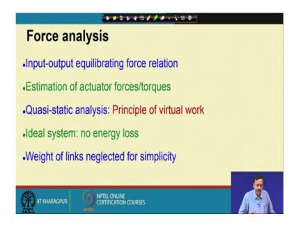
So, under force analysis, we are going to look at the input output equilibrating force relation. This will give us an estimation of the actuator forces or torques that are required that will be required.
