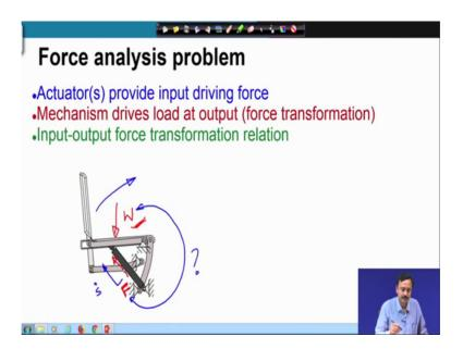
So, what is the force analysis problem? So, as I have mentioned the actuators provide input driving force, the mechanism drives certain load at the output and the force can get
