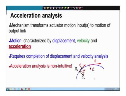
Let us review the things we had discussed before we know that a mechanism transforms the actuator input motion to the motion of the output link. Now motion as we know is characterized by displacement velocity and acceleration and in these lectures, we are now discussing the acceleration part. We have already discussed the displacement and velocity analysis of mechanisms and robots.
