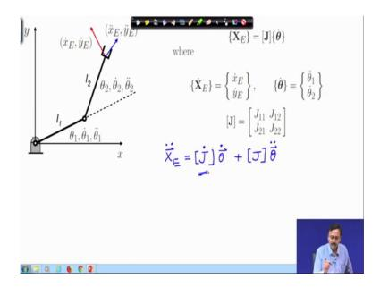
Now, if you differentiate this velocity relation with respect to time as we have been doing. So, we will obtain xE double dot is equal to the time derivative of the Jacobian remember that the Jacobian is a function of the configuration. So, time derivative of the Jacobian times the joint velocity vector plus Jacobian matrix times the joint acceleration vector. Now this Jacobian derivative is now a little more complicated.
