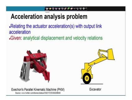
So, the acceleration analysis problem is about relating the actuator acceleration in input with the acceleration of the output link. And we are given the displacement and velocity relations. So, we will start with these as inputs.
