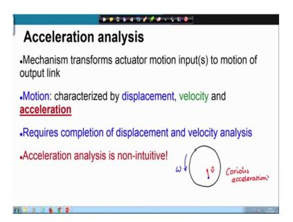
And that is of a disc that is rotating at a constant speed and a particle that is moving with respect to the disc also at a constant speed let us say.
