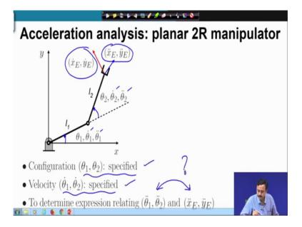
Next let us look at the acceleration analysis of a planar 2R manipulator. So, here I have shown a 2R manipulator which is moving at a certain configuration it is moving with
