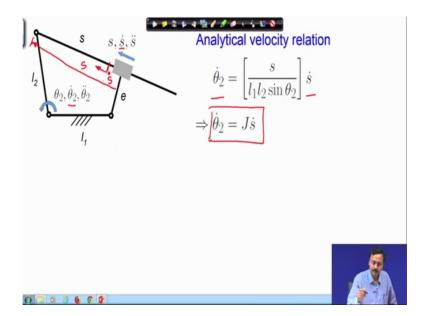
So, we will start off with the analytical velocity relation which we have derived earlier further for this chain. I have mentioned that this is the angular speed at the output link and the angle and the linear speed at the input of the prismatic pair.
