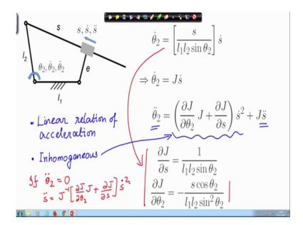
So, let me rewrite these expressions and determine what is del J del theta 2 and del J del s. So, these are the relations which can be easily obtained from here by differentiate differentiating with respect to s, I have del J del s and with respect to theta 2 I have this expression of del J del theta 2.
