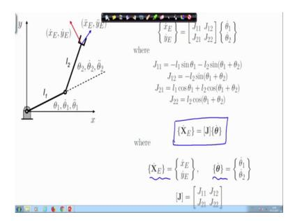
This can be written in a compact form as shown here, where xE dot this is the end effector velocity vector and this theta dot vector is the joint velocity vector.
