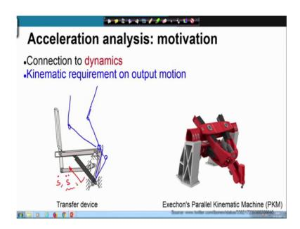
Now, the motivation for; that means, doing x acceleration analysis is that it is connected to dynamics. For example, Newton's second law relates the acceleration of a particle or a rigid body center of mass of a rigid body to the forces acting on the particle of the body. There is another requirement that we have and that is the kinematic requirement on the input output motion.
