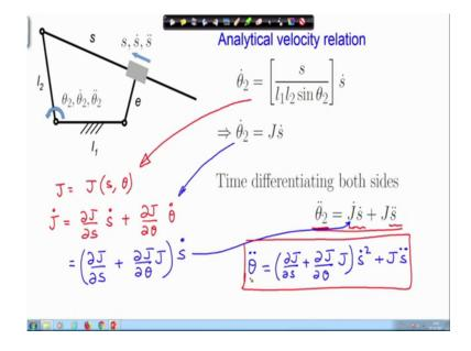
So, if you differentiate with respect to time both sides of this velocity relation you will obtain this acceleration relation. So, on the left I have the acceleration at the output and on the right, I have a term where I have the time derivative of the Jacobian and the rate of expansion of the actuator; and a term which involves the acceleration of expansion of the actuator.
