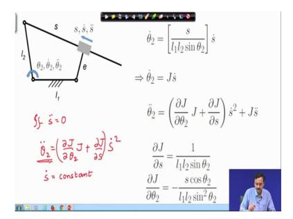
Similarly, if I have the input as a constant which means if s double dot is 0; that means, that prismatic actuator is expanding at a constant rate; in that case I have acceleration at the output. If I am moving at a constant if I have the prismatic actuator expand at a constant rate which means s dot is constant, then the output has a angular acceleration.
