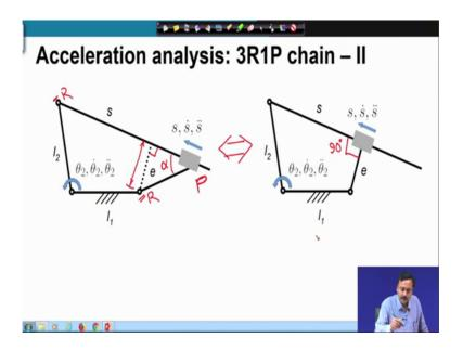
So, this is the distance between the 2 revolute pairs connected to the ends of the links with the prismatic pair. So, here we have the prismatic pair and these are the 2 revolute pairs connected to the links which are connected through the prismatic pair. So, the distance between these 2 revolute pairs measured in a direction perpendicular to the direction of the P PR is the offset now this angle let us say alpha is a constant.
