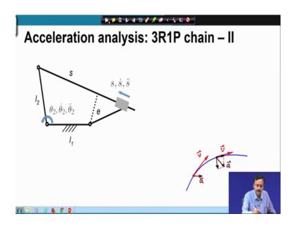
We will start with the acceleration analysis of a 3R1P chain of type 2, we have discussed this point before that for a 3R1P chain of type 2 here we have the offset.
