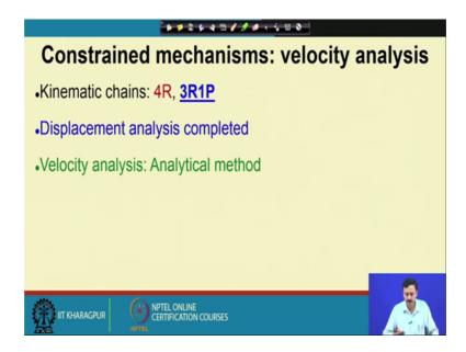
And we are going to look at the chain, we will consider that this displacement analysis is completed which means that we know the configuration of the mechanism. As you know in constraint mechanisms specifying one of the input one input will specify the configuration of the complete mechanism so, I can find out all other angles. Am angles and of course, the throw of the prismatic pair. So, here in the we have a prismatic pair. So, we can calculate everything given an input.
