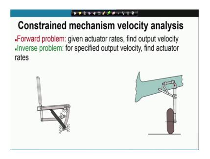
We have these problems for the constraint mechanisms.
