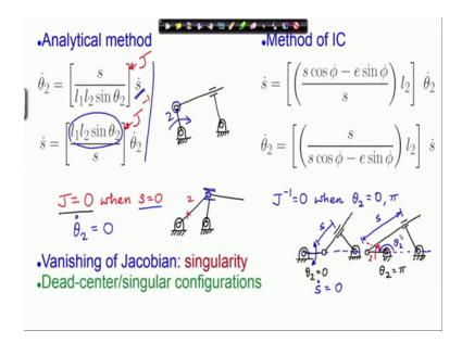
So, this these are the expressions of the velocity relations obtained from the analytical method and on the right, I have written out the velocity relations obtained from the method of ICs.
