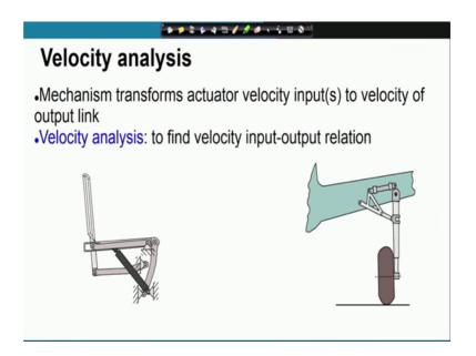
So, the velocity analysis problem has been defined as the as finding out the input output velocity relation; that means, from the actuator to the output.
