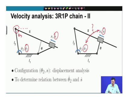
So, the configuration of the mechanism is known to us, which means theta 2S and also this angle theta 3 of course, these are all known to us theta 2S theta 3 these are all known to us from displacement analysis. We have to find out the relation between theta 2 dot and s dot. So, we have to find out this relation.
