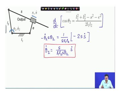
So, this is the displacement relation, so what do we have? Minus of theta 2 dot into sine theta 2 is equal to 1 by twice of 11 l2 times. Now these are constants l 1 is constant l 2 is constant. The only thing variable is S, e is a constant. So, this is as simple as that. So, therefore, I can relate, let us say theta 2 dot as like this.
