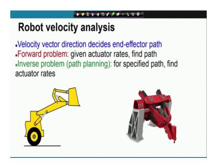
For robots, in which the path planning problem or path generation problem is of importance and which were intimately depends on the velocity analysis problem for robots.
