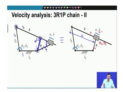
Now, in the chain of type 2 we have a prismatic pair which is changing the direction of the sliding as you can see here. As we have discussed before, you can see that this angle is going to remain fixed. When the prismatic pair expands or contracts so, to number the links the ground is 1, this is 2, this is 3, this is 4.
