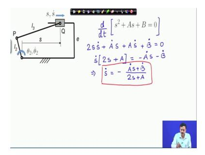
In terms of A and B which are functions of theta 2. So, if I take time derivative of this expression, what do I have? I have 2 s s dot this is d d t of s plus e dot s remember A is
