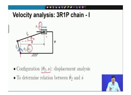
So, this is the 3R1P chain type 1. As I have mentioned that the configuration in terms of theta 2 s and also of course, theta 3. So, if I know theta 2 for example, I can find out s I
