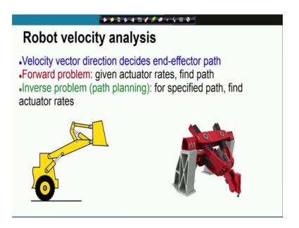
And for robots we have the path planning problem, which is the inverse problem which is very useful for in a generation of output trajectories by a robot manipulator which we were going to discuss very soon.
