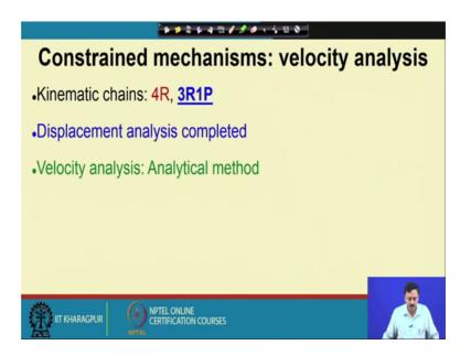
So, in this lecture we are going to look at the 3R1P chain of type 1. We will assume that the displacement analysis is completed, which means that I know the configuration of the mechanism of course, I am given one input because this has one degree of freedom I can calculate the other angles using the displacement relations. We are now going to embark upon the velocity analysis problem.
