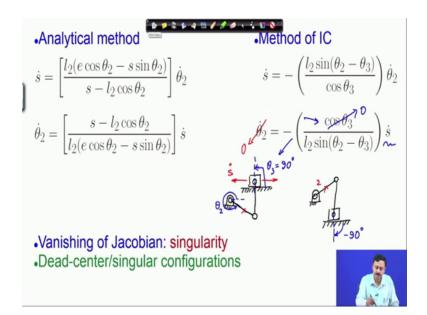
So, the Jacobian becomes singular at this these 2 configurations and therefore, these are the dead center configurations of the mechanism, there is another set of dead center configurations which we have also looked at just to reiterate the point. So, here this is theta 2 and this angle theta 3, this 90 degree what happens that when theta 3 is 90 degree as you can see here cosine of 90 degree is 0.
