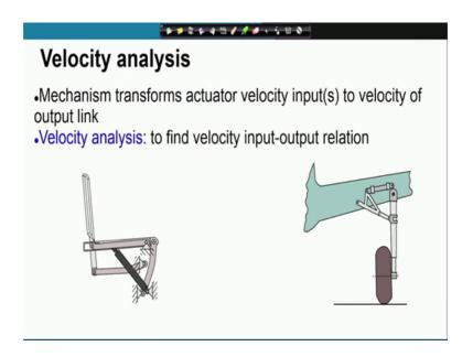
So, we have looked at the velocity analysis problem before so, will quickly go through that. So, essential goal of the velocity analysis problem is to find out the velocity input output relation, and the inputs are the actuators, and the output is the is a it can be a link or the end effector of a robotic manipulator.
