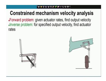
So, in the case of constraint mechanisms you have just 1 output link, and corresponding to an input velocity we have to find out the velocity of the output link. So, you have the 2 problems forward and inverse, given the actuator rates finding out the output velocity is the forward problem, and for a specified output velocity finding out the actuator rates is the inverse problem.
