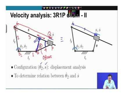
So, here is the 3R1P chain type 2 here we have the angle theta 2, and S this variable S is this length is s. So, this is the expansion of the prismatic actuator. So, here we have the prismatic actuator. So, S is the length of expansion of the prismatic actuator, previously we had defined this offset e which is measured in the direction perpendicular to the direction of the prismatic pair. So, this is the direction of expansion of the prismatic pair or motion of the prismatic pair.
