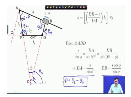
So, S divided by sin of this angle phi is equal to D A divided by sin 90 degree, this angle is 90 degree. And also equal to D B divided by sin of 90 minus phi. So, if this is phi this is 90 so, this must be 90 minus phi. So, that implies D A is equal to S divided by sin phi and D B is S cosine phi divided by sin phi.
