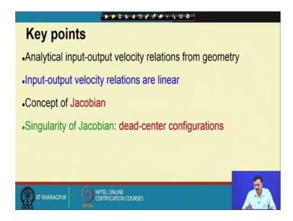
Velocity relations from geometry which are linear, the input output velocity relations are linear. We introduced the concept of Jacobian and we have looked at the dead center configurations of the mechanism.
