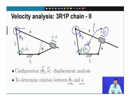
I can also find out this angle which is theta 3 or in this case here. So given theta 2, I can find out using displacement analysis S as well as theta 3, or I might be specified S then
