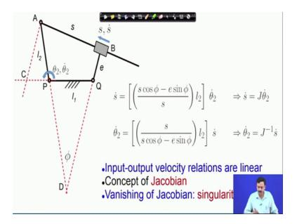
What is the other situation? The other situation is the other singularity is when the Jacobian inverse. So, this is Jacobian inverse so, Jacobian inverse vanishes when S equal to 0, and when can that happen at this configuration something like this. So, here S equal to 0, and that is the singularity where theta 2 vanishes irrespective of value of S dot. So, these are the 2 singular configurations, which I have written out for you.
