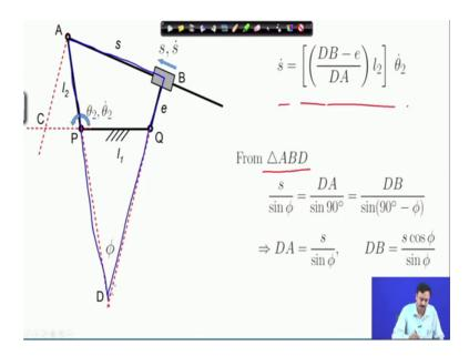
So, I have again written out that expression of S dot relating the theta 2 dot as I mentioned D B and D A are as yet unknown. Let us look at this triangle A B D. So, A B D so we are looking at this triangle A B D so, using sin rule I can easily write S divided by this angle sin phi sin of this angle.
