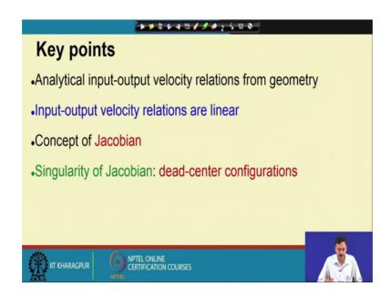
So, let us recapitulate the key points, we have found the analytical input-output velocity relations from geometry. Now, here I must mention again that we have used the concept of instantaneous center of rotation of the mechanism and then from geometric relations we have tried to find out certain lengths.
