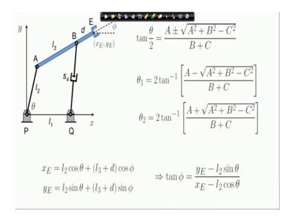
So, from here I can solve for phi; again using the A tan 2 function because I need to get the quadrant right.
