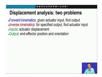
Now we have two kinds of problems as you know the forward kinematics problem in which the actuator inputs are given we have to find out the output; output is the end-effector position or position and orientation depending on degree of freedom of the chain.
