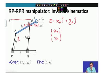
Now, let us move on with the. So, this is the RR RPR manipulator and we are going to study the inverse kinematics of this chain.
