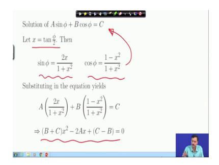
We will take this approach which can be very easily programmed on a computer and you can get all the solutions of this equation A sine phi plus B cos phi equal to C. So, in that we make a definition x equal to tan phi by 2 and represent sine phi and cosine phi in terms of x which when substituted into our master equation finally, gives us this quadratic equation in x whose roots, we can now easily find out and hence we can find out tan phi by 2 and that is what we are going to do.
