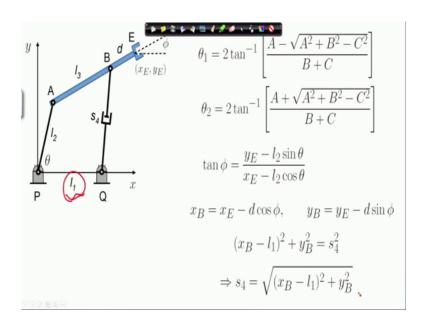
So, from here I can find out the throw of this prismatic actuator. So, this is what I have written out. So, S 4 is square root of x B minus 1 1. So, you have I one here the length P Q. So, x B minus I one whole square plus y B square because y Q is 0 the y coordinate of point Q is 0.
