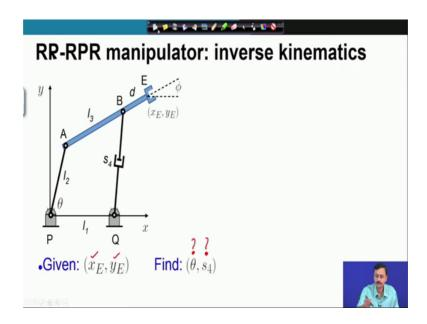
Now here we are given the coordinates of the end-effector and we are to find out the inputs; the actuator inputs which are given by theta and S 4. So, here I have written out.
