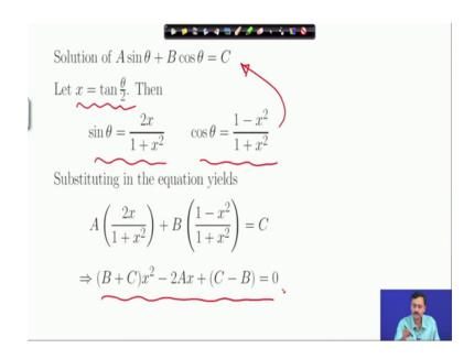
So, once again just to reiterate what we have done we have defined this x in terms of tan theta by 2 express sine theta and cosine theta in terms of x substituted into the equation that we want to solve and finally, obtain this quadratic equation which has solutions in terms of A, B, C which are completely known to us we have 2 solutions as you can see again here.
