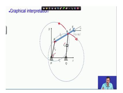
The solution graphically remember that we are given theta and S 4. So, therefore,. So, theta and S 4 are given. Now if you see when theta is given then this point A gets fixed what is not fixed is phi because this hinge be on the end-effector link can rotate on this circle while the hinge be on the actuator arm on this other leg can rotate on this circle.
