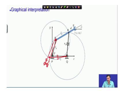
So, you have one configuration that is already shown there is another solution, this is given by this your hinge B can also lie here. So, therefore, the mechanism in this configuration will look like this. So, in the red configuration because point A is fixed remember because theta is given since theta is specified a gets fixed and hence you have another assembly mode of this mechanism as shown by this red configuration. So, these are the 2 solutions.
