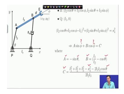
Some A sine phi plus B cosine phi equal to C which you can easily do where you will find that this A, B and C are completely known because I know theta and I know S 4. So, therefore, A, B and C are completely known to me; so, what is unknown is phi which I need to solve from this equation.
