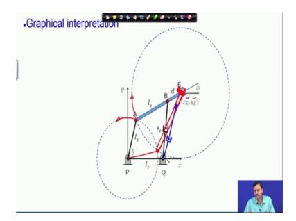
So, let us understand this solution graphically we have been given x E and y E. So, this point E is fixed what is not fixed is this hinge a on the end-effector link a can move on this circle on the hinge on the link 1 2 can move on this circle. Therefore, if I want to assemble the mechanism then it can happen only at these intersection points of the two circles.
