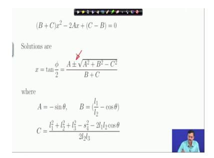
So, the solution solutions of this quadratic equation you have these two solutions given by these 2 signs positive and negative. So, we get two solutions of x and hence two solutions of phi A, B and C are completely known.
