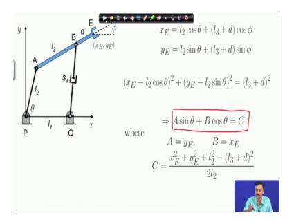
The forward kinematic solution you remember we are derived these expressions of x E and y e. So, we start with the forward kinematic solution or relations if I take this term.
