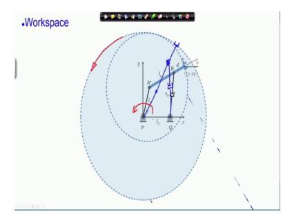
So, if you completely extend this link and then move it in the circle; you generate the outer circle which defines the workspace of this manipulator. Of course, with joint limits or actuator limits this workspace is going to get more complicated and will be reduced which you can find out based on geometry.
