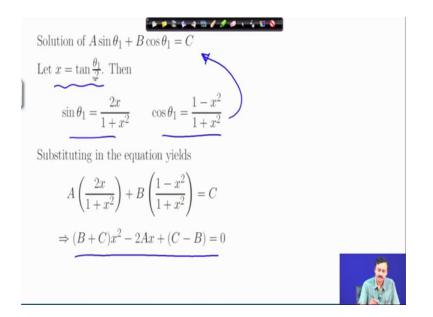
So, let me show this solution of A sin theta 1 plus B cosine theta 1 equal to C. So, we have followed this procedure, many times we make this substitution, we redefine redefine this variable x and x plus sin theta 1 plus cosine theta 1 in terms of x, which when substituted in the master equation gives us this quadratic equation, whose roots give us tan theta 1 by 2.
