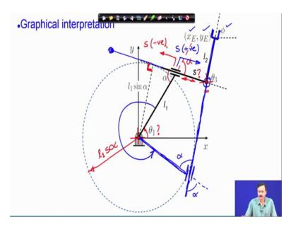
We will understand this for an arbitrary angle alpha as I have shown here. Now what is specified to us is xE yE and phi these are specified. So, once these three things are specified, this length gets fixed, this link gets fixed. So, which means this kinematic pair is now fixed, this is the ground joint, ground hinge. So, that is definitely fix. So, these two are fixed. Now what remains to be found, is this angle theta 1 and just throw of the prismatic actuator which is S.
