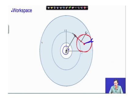
And the farthest reach is when you have, this comes here this revolute pair and you can generate a full circle. So, this is the third link of the manipulator. So, this is the farthest reach, and now if you rotate this angle then you sweep on the outer circle.
