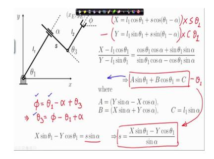
Now, in order to solve for S, I have multiplied the first equation by sin theta 1, the second equation by cosine theta 1 and I have taken the difference. When I do that on the right hand side I am left with only S sin alpha therefore, to solve for S I just divide throughout by sin alpha. So, this is my expression for S. Now, therefore, our solution procedure, is first find, first solve for theta 1.
