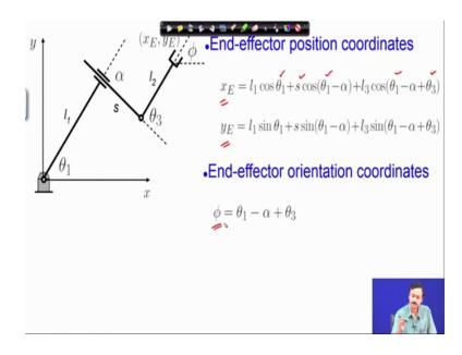
So, xE yE expressions and finally, the end effector orientational coordinate. So, which is phi. So, this is the forward kinematics problem. So, given theta 1 theta 1 S and theta 3, I will be able to find out xE yE and phi.
