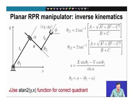
So, theta 1 has two solutions. Once again this tan inverse you have to use atan 2 function to get the correct quadrant. So, we have two solutions of theta 1, theta 1 and theta 1 2. S is obtained in this form which we have derived. Finally, we have theta 3 which can be found in terms of phi and theta 1 and alpha is a fixed angle. So, this completes the solution for the inverse kinematics problem.
