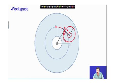
Now, the workspace, here you can see that this prismatic pair will rotate on this circle. So, therefore, this sliding ring sliding element will always be moving in this direction, in this particular case with alpha is 90 degree this will be tangent to the circle. If this angle is 90 degree then this link moves tangent to this circle. Now this revolute pair can rotate; therefore, this describes the circle.
