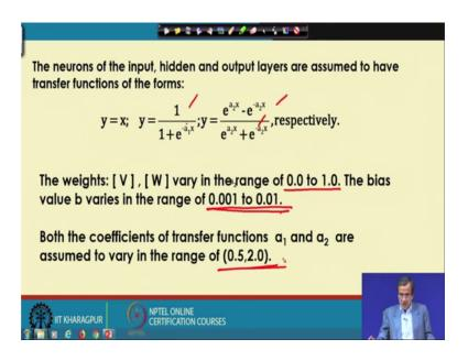
Now, as I told that input layer we have got the linear transfer function and on this hidden layer we have got the log sigmoid and on the output layer we have got the tan sigmoid transfer function. The connecting weights V and W those are lying in the range of 0.0 to 1.0 and the bias value we are varying in the range of 0.001 to 0.01. So, this is the range for the bias value b these are the range for the connecting weights 0 and 1, and these are the transfer function.
