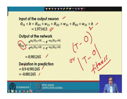
So, using this we can find out the output of this hidden neuron like H O1, H O2, H O3 and once we have got the output of the hidden neuron. Now, I can find out the input of the output neuron. So, the input of the output neuron that is O I1 plus b is nothing, but H O1 multiplied by w 11 plus H O2 multiplied by w 21 plus H O3 multiplied by w 31 plus b. And if you substitute the numerical values, so you will be getting, this is actually the
