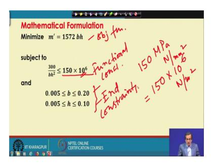
So, very easily we can mathematically formulate so, this particular optimization problem. So, our aim is to minimize m prime that is the mass of this particular cutting tool and that is m prime is 1572 bh subject to the developed bending state that is 300 divided by bh square is the less than equals to the allowable that is 150 raised to the multiplied by 10 raised to the power 6.
