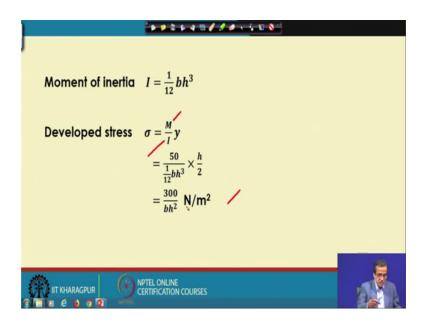
Now, once you have got the moment of inertia expression the develop stress that is nothing but the bending stress, now bending stress we know the formula like the first year mechanics the bending formula is M divided by I into y M is nothing, but the moment M is nothing, but actually the maximum bending moment I is the moment of inertia and y is nothing, but h divided by 2 that is the half of this particular height that indicates actually the location of that particular the centerline.
