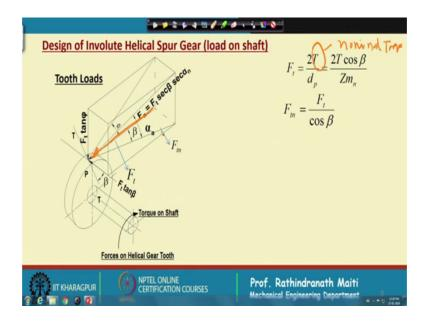
Now, we shall consider what is the tooth, what is the load coming on the shaft from the gears? Now first of all we will calculate the tangential load F t is equal to twice T divided by pitch circle diameter which is twice T cos beta divided by Z into m n.
