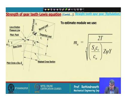
Now, in the figure, it is shown a tooth is subjected to load; this means it is transmitting torque the torque gives the tangential load; that means. So, this tangential load is directly derived from the torque divided by the radius. As earlier specified; this tangential load is actually acting at the pitch circle, it is somewhere here at acting at the say here acting at the pitch circle, but while we are designing the teeth; we consider that as if the tooth is acting at the teef.
