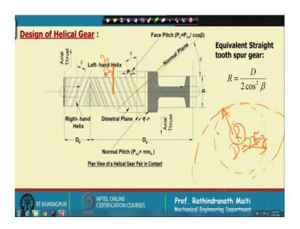
Now, if we come to the helical gear this helical gear we may consider the straight tooth spur gear a in they are very thin straight tooth's Spur gear, they are put together one after another with a slight rotation. So, if we consider say let us consider this. This is the gear and this is the pinion and these are straight teeth not the helical which is shown in this figure.
