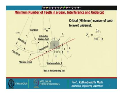
Now, this is already in earlier lecture I have shown that what should be the critical number of teeth to avoid undercut this is given by Z c is equal to twice into addendum factor divided by sin square of this standard pressure angle. Even if we use there the gear
