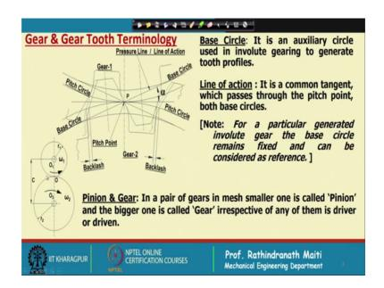
Now, if we consider the involute gear teeth, then as already discussed this is we can consider a cross belt drive and if we take a point on the cross belt drive that generated the involute profile, and on to drum we can set that profile and we can replace the belt. Now the question is that how to maintain the continuity in the motion for that we must have these profiles at a certain interval and when one profile is going out of touch, then another profile should come into contact.
