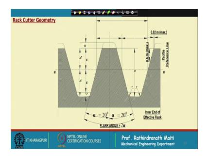
Now, this is again the proportion of a standard rack cutter these all these dimensions will be given when this rack cutter is selected and from we must know this geometry to find out the actual profile of the teeth.
