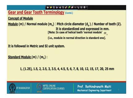
Now, we shall learn a little bit about the other terminology. Now first of all the module already I have discussed, but the module is this expressed in millimeter the module into the number of teeth will give you the pitch circle diameter of the gear. Now as I told the pitch circle again, when the gears are meeting, if the center distance are different then definitely there will be change in pitch circle. Then what we should call the pitch circle of a gear?
