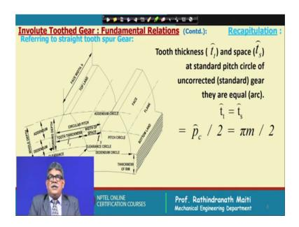
Now, tooth thickness arc tooth thickness and space arc space thickness, you can call at standard with circle of uncorrected or standard gear they will be equal; that means, d t cap is equal to t s cap and both are equal to the circular pitch divided by 2 that is pi m by 2.
