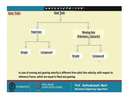
Now, considering the gear train first of all gear may be fixed axis, gear means gear unit, there will be pinion and gear may be in a single stage or stages may be two, three etcetera, etcetera. In fixed axis, first of all you will find the simple. Simple means in this case you may consider one pinion and one gear.
