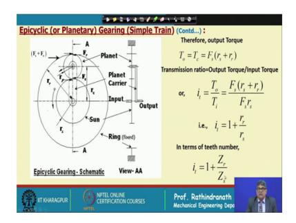
Now, therefore, the force F s is equal to r s plus r r. And therefore, the transmission ratio the T output divided by T input which is F s by r s by r r divided by r s the radius of sun, the radius of ring plus radius of sun divided by radius of sun that means, it will become 1 plus r r by r s.
