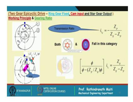
And from there we will find the transmission ratio, this is i 2 we have designated at 2 because we are keeping this ring gear fixed and we get minus Z p by Z g minus Z p. If we equate the earlier one, if we equate this one, we will arrived into here. Now, this the two gear epicyclic later we will show that can be put into where this is a another special gear the same principle it is working on the same principle.
