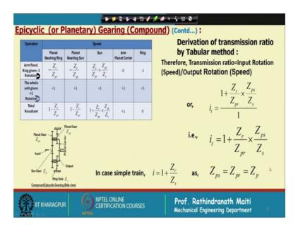
Then from this table, we find out that the transmission ratio is the input rotational speed divided by output rotational speed in terms of torque, these are otherwise output torque divided by the input torque. But in this table, we have found out the motion. So, according to that this output say input motion input speed divided by output speed that means rotation not speed because we have not considered the time part.
