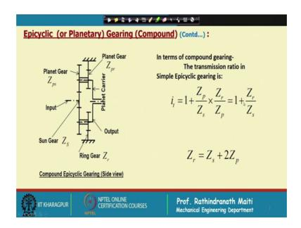
So, this is the compound gear, it is shown like it is the side view is shown here. This is the sun gear and it is mating with the planet gear teeth number of which is given by Z ps. And then on the same shaft, there is another pinion which is of smaller diameter and than this one and the teeth number is given by Z pr and this is the ring gear.
