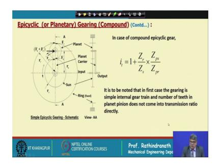
In case of compound gear, which is not shown here, this is the this is not the compound one, this is the simple one. In case of compound one this will be Z r into Z s into Z ps by Z pr that means, this is the here now there will be two gears we will show see into the next slide.
