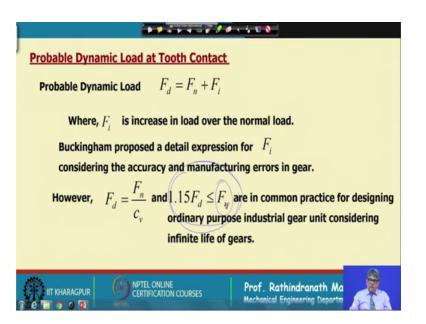
And then so, this is the formula already discussed and then that would be considered, that would be compared with the Probable Dynamic Load. Probable dynamic load will be the it is a it is usually normal load acting and the teeth plus some increment and the load due to the dynamic effect. So, that is given F n by F i there are various formula proposed by various gear researcher.
