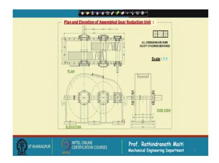
But, one thing you should remember if we go for say for example, if you take the first stage bevel second stage helical, then in that case it is better we should go for taper roller bearing. So, that shaft does not move this way or that way, because of the reasons contact of the bevel gear depends on do not allow the movement of the shaft in axial directions we have to keep it form. So, you will find normally that is with the taper roller bearing.
