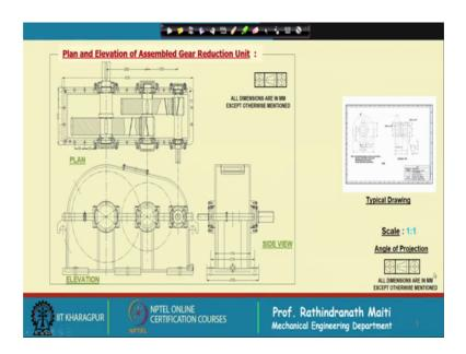
Now, this is the view plan view elevation and side view although not completed, but the gearbox what we have designed in the last page that is considering total reduction ratio 24.42 keeping the input shaft and the intermediate shaft same only the output gear had changed, for that the gearbox will look like this. And I would say this gearbox with a little refinement here and there can be seen for manufacturing ok.
