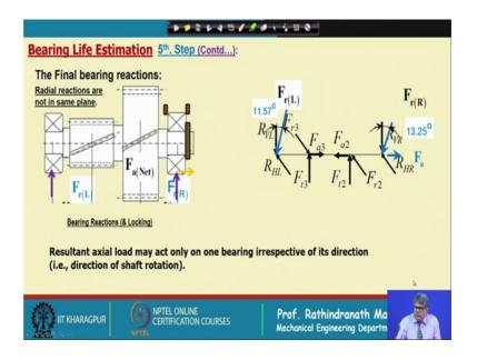
And, then only you can calculate what will be the load coming on the bearing, because now you can calculate from the torque what is the load acting at the contact points? And from there as you know the bearing distances and distances from the mid of the gear a mid of the pinion two different bearings, you can calculate all these loads ok.
