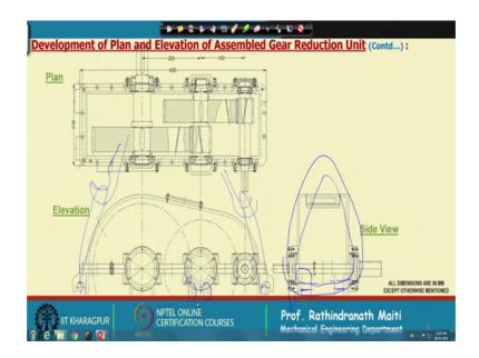
Now, if I in this view what we have done I have shown the elevation not fully bottom portions just to show you that, this covers we have 6 bolt 1 2 3 4 5 6 bolt this is also we have taken m 5. Now, here this bolt is simply tightened on the bearing seat there will be scaffold. And, if we look into this view here say here this is these are the 6 holes for tightening the cover m 5 bolt and thread is made inside this housing raised portions where the bearing are settled.
