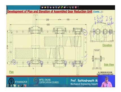
So, this means that if we look into this here there will be 1 bolt, 1 nut and 2 spring washer one at the top and one at the bottom, but sometimes we can use one side plane washer other side spring washer, but better to put with the spring washer. So, that it will not easily open due to the vibration ok.
