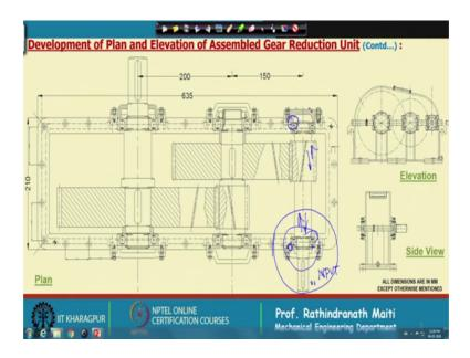
Now, this is in this view what I have shown the, we have zoomed out that the plan view of the gearbox. Now, if you look here in this plan view first of all this is I have already shown this part, that is the input shaft this is input shaft sorry this is input shaft and in the input shaft, what we have put who we have put the cover and oil seal we have put the cover and oil seal, which is shown already shown in the previous lecture.
