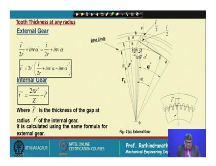
Next, if we consider this geometry, we have considered a full teeth, we have considered a full teeth and we have shown here that this is equal to involute alpha dash; that means, or this angle total this plus this is phi or phi angle from this line to this line ok. So, that is nothing, but involute alpha dash.
