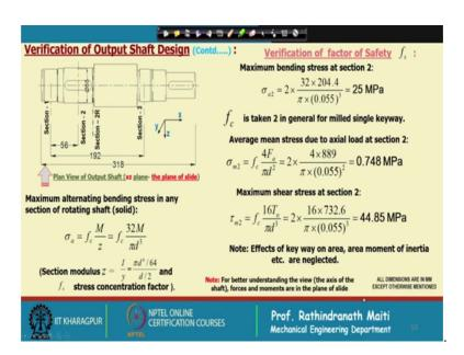
Now, the verification of the factor of safety in that case we know this formula the sigma a is equal to M by z z is the section modulus more popularly M y by I and f c is a factor that we have multiplied with to calculate this frictional stress.
