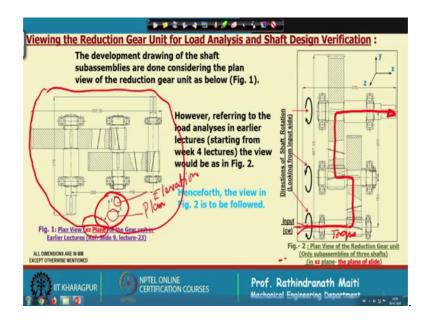
Now, another issue I would like to discuss. Now I axis system is shown this is the axis system. So, this is the axis system x y and z ok. And as you see this figure drawn here it is in x z plane, because this is we have developed the plan view. So, it is in that plane now; that means, this is for plan and this is for y x will be elevation.
