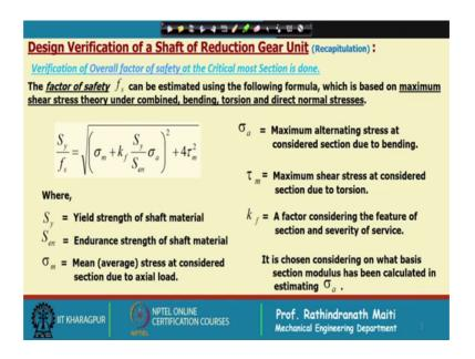
Make next verification of overall factor of safety at the critical most section is done; that means we will do that. Now first of all if you remember that in week 4, we verified the design of the intermediate shaft. We also very I mean we verified the factor of safety there, the same way we will we shall verify the factor of safety here also.
