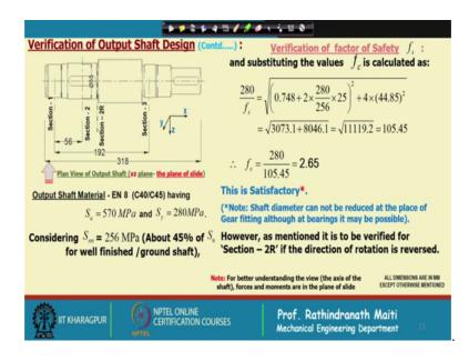
So, material of this shaft is EN 8 that is C 40 or C 45 according to Indian standard EN 8 European national standard and for which the endurance strength we can consider. If it is
