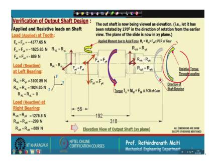
Now, this again if we look into this that now we have taken the elevation part. Elevation part means we are looking the gear everything from the z direction and putting into the x y plane ok.
