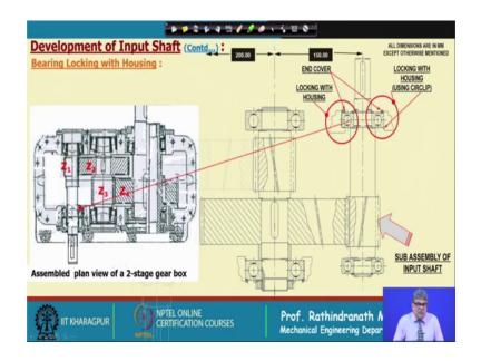
Now, we will think of the locking with housing. Now, here as you see, has already described. We can use is circlip for locking the inner end of the bearing, if we, why we are trying to lock this, this end bearing, because as the pinion is closed to other end bearing, that will have the maximum load radial, loads here, the radial loads will be less. So, what we can do? We can lock this bearing fully.
