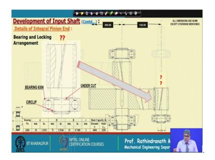
If we look into the developed figure of that, there is the , this portion I have shown in the developed form and this is the bearing and this is the circlip and one mistake is there in the pinion and the intermediate gear. There is two centre lines, but there will be only one
