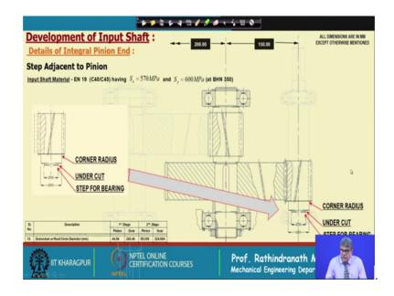
Say we developed this much earlier and next, we are, developing the input side of this shaft. Now, this is the material, is shown as well as that, what is the denim circle, that is also shown and it is shown the input portion of the pinion and then there is a step and then the, we are, we are gradually, we shall develop the, seat for the bearing, this is, this is the pinion end, other side will be the input end.
