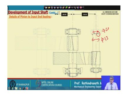
So, we need not put any other special or anything the bearing, inner race can directly rest on this solder of the step here, it can stave. So, rightly this is around 43 and here it is around 30. So, this means that we will have 13 millimetre. So, 13 half of that 6.5 millimeter is good enough for taking load through, in a race of the bearing now.
