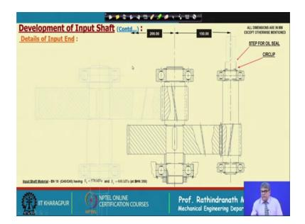
Now, next stage, we major that this for stiff for oil sealing. We are keeping around 12.5 millimetre have about half an inch and usually this while, since our seal of 30 diameter will have an thickness of 8 millimetre or; so, assuming that and after that there will be space for the cover material, we have made it like this and then the shaft diameter is further reduced for input; that means, a coupling to be fixed.
