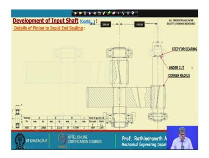
So, again we have the corner radius here, as shown. This is the corner radius that corner radius is given due to this corner radius and edge. This diameter is very close, you an impression of gear cutting may be evident, maybe it will be prominent on that corner also, but it does not matter it will make no harm of the shaft.
