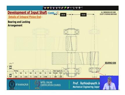
Now, bearing and it is locking arrangement. So, bearing selected already we, I have shown, but here it is also displayed, what is the capacity of the bearing and size and then we place the bearing ok, and that bearing is locked with a circlip and we.
