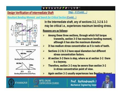
Now, in earlier in previous lecture I have already shown that how to calculate bending moments at two planes. And in this figure it is shown on the shafts in two planes what
