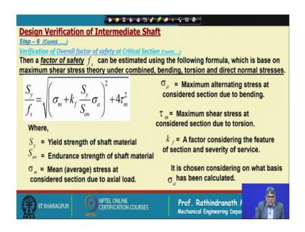
Then what we do a factor of safety can be estimated using the following formula which is based on maximum shear stress theory; under combined, bending, torsion and direct normal stresses. The formula is proposed here it is not proposed I would say this is a modified form of maximum shear stress this stress formula which is subjected to bending moment and the torsion.
