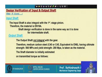
Now, if I consider the input shaft this is also designed in the same way; that means, we have to calculates calculate all loads on the bearings from their bending moment, we have to select the critical section also that is shaft is also having the pinion integral and,
