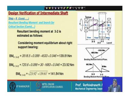
Now, for the section 3-2 first of all again from the moment calculation; so, we need to calculate because from the graph of course, we can take we can measure, but we separately we calculated calculate it for section 3-2 that is from the left hand load to this distance of this section which is 0.099 meter and minus the load acting at the pinion into the distance up to that point.
