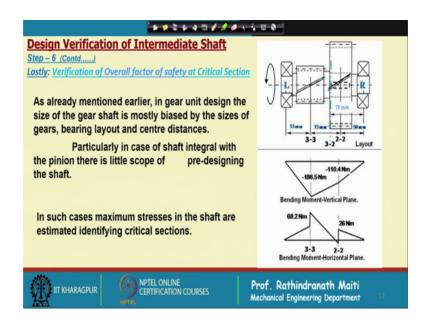
As already mentioned earlier in gear you need design the size of the gear safety is mostly based on by the size of the gears bearing layout and centre distance. Particularly in case of shaft integral with the pinion there is the there is little scope of redesigning the shaft.
