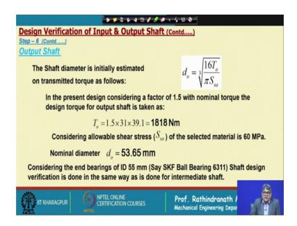
And in the present design the factor of 1.5 with nominal torque the design torque the output shaft is 1.5 into 31 because in designing shaft we have considered the input torque is 31 and the total transmission ratio is 39.1. So, torque is 1818 Newton meter and the shear stress of selected material is 60 mega Pascal, nominal diameter is 53.65 millimetre.
