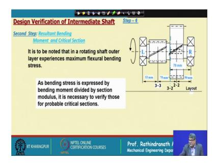
Now it is to be noted that any rotating shaft, outer layer experiences maximum flexural bending stress. As bending stress is expressed by bending moment divided by section modulus it is necessary to verify those for probable critical sections.
