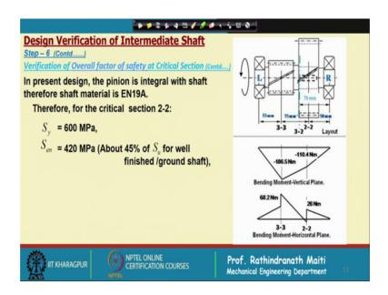
In present design, the pinion is integral with shaft therefore, the shaft material is EN19A which is the material for the pinion. Therefore, the critical section 2-2 for that critical section we will consider the yield strength is 600 mega Pascal which is given, endurance limit is 420 mega Pascal which is if not given can be taken as 45 percents of the ultimate strength for well finished and ground shaft; shaft may be ground if it is heat treated after the gear hobbing.
