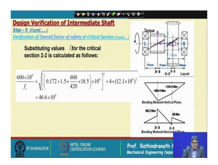
Now, the mean stress due to the axial load is simply may be taken at that section; at the section 2-2 is the axial load because axial load is acting there very much because our axial load is going to the right bearing therefore, at section 2 definitely the axial load is there.
