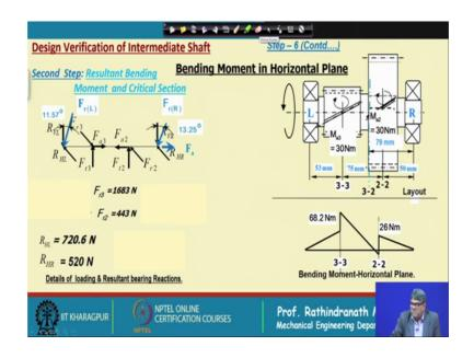
Now, we shall consider the horizontal plane also in horizontal plane what are the loads? You can find out the loads here in the horizontal directions.
