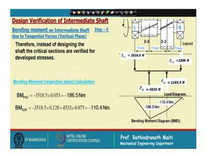
And, similarly for vertical plane we calculate also the shear force sorry we calculate the bending moment diagram. In the bending moment diagram again as it is bending in the upper directions; we draw the bending moment in these directions and these are the bending moment at these two sections. We have considered these two sections as there are bending moments are changing.
