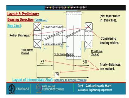
Now, this is the intermediate shaft of our gearbox what we have designed we have taken the module in first stage 3 millimetre and in second stage, it is 4 millimetre. So, this is this is the fastest gear and this is the second stage pinion. Now, we will see that this is the layout is made and from there we have considered this shaft.
