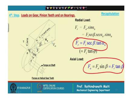
So, if r radial load on the gear finally, can be expressed as F t sec beta sec alpha n and sine alpha n or simply F n sine alpha n and sorry this actually F t 10 psi which is also can be given I, this angle is I also can be given usually better to use this formula F r is this one this is helix angle this is pressure angle whereas, for axial load we use this one it is clear that if the helix angle is 0, then axial load will be 0.
