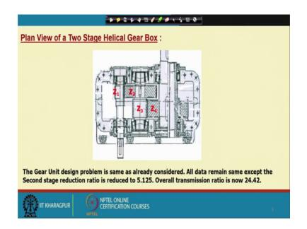
Now, the what the problem we have taken we are going to design a two stage helical gear box which looks like this what is shown. This is the plan view, top open plan view of the gearbox. And z 1, z 2, z 3, z 4 are the teeth numbers. In first stage pinion teeth number is z 1, and gear is meeting gear is teeth number is z 2. And thus in second stage pinion teeth number is z 3 and final output through the meeting gears z 4.
