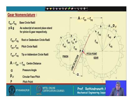
Now, at such the nomenclature of gear which earlier shown, the here it is a meeting gears is shown. Pinion and gear both are shown; and line of action also shown with a pitch point. And most of the dimension will repair for the drawing. However, the base circle which is designated by r b, r b, e pp and r bg, where p stands for pinion, g stands for gear.
