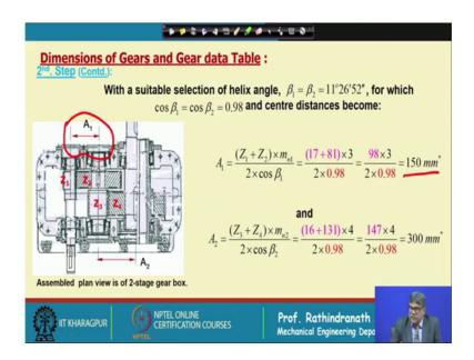
And then, we calculate the gear data or gear dimensions these are in the tabular tabular form. This with the drawing and also the below material this data is provided. This is for the manufacturers and as well for also for further design, what we find the 1st stage pinion is pinion teeth number is 17 and gear is 81, 2nd stage 16 131. Pressure angle 20 degree a stage module 3 mm, 2nd stage module 4 mm, and helix angle both are same for both stages which is 11-degree 26 minute 52 seconds.
