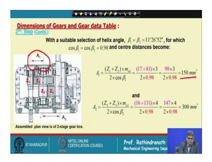
Now, helix angle, Helix angle we have considered it is 12 now, if we give this is 12 then, the factor at the denominator that cos beta which is coming into the pitch circle diameter as well as, in the center distance. We will find that number and that that value will be a fraction, which is not desired. It is to be mentioned for standard gearbox.
