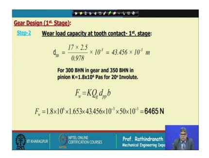
Now, dpp that is pitch diameter of pinion is 17 into 2.5 divided by cos beta we have considered helical gear. So, we have taken 0.978 into 10 to the power 3, which becomes 43.456 into 10 to the power minus 3 meter . That is, it is 43.456 mm. For 300 BHN and in gear and 350 BHN in pinion, K it can be taken as 1.8 into 10 to the power 6 pascals for 20-degree involute. This is from available data in machine design books or design data book.
