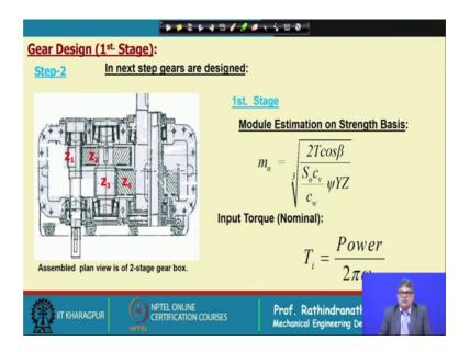
Next, we shall consider the design of gears. Now, first stage if we consider the formula it is modified Lewis formula for bending strength. We find this module can be estimated by considering the torque helix angle and alloy will strength of the material, width factor, form factor and the number of teeth. We have consider the helical gear, so, we will now consider the other values.
