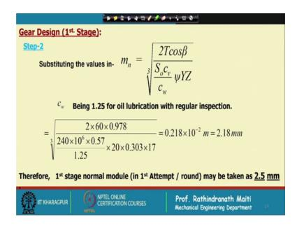
Now, with this value and c w we have considered 1.25 that oil lubrications with regular inspection this means that inspection will be regularly, but not may not be very frequent and it is in oil some the gears are in oil some that is just (Refer Time: 26:40) lubrication we have consider this value is 1.25.
