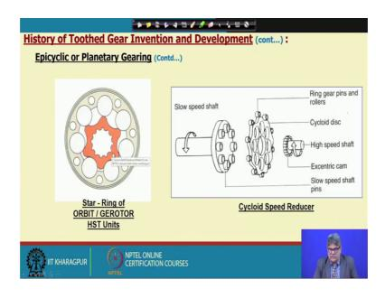
So, this gives also the gearing motion and with the same profiles that is a epitrochoidal profiles the gear unit is also available which is called cycloid speed reducer as you see here this is the epitrochoidal star and these are the loabs in the envelope which is essentially circular and the planet this is the input this is a cam sort of thing eccentric cam and the output is taken through these holes with the planet carrier.
