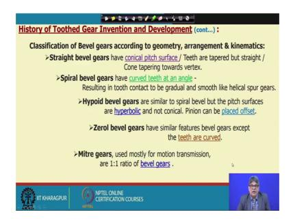
Now, here it is perhaps we should know particularly bevel gears they are of various type the street bevel gear which I have shown in earlier slide, it has the conical pitch surface teeth are tapered, but straight and cone tapered tapering towards vertex.
