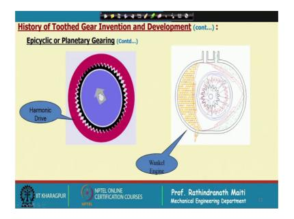
Now, then we I shall discuss about some very special gear, in this special gear, what we find? The outer ring gear is fixed and a in pinion, it is moving apparently, it is flexible, yes, it is a flexible gear and hear the tooth difference is only true and we get the reduction in the order of the tooth number of the ring gear divided by two or tooth number of the pinion divided by two depending on which one is fixed; fixed mean rotation of it is about it own axis is restricted ok.
