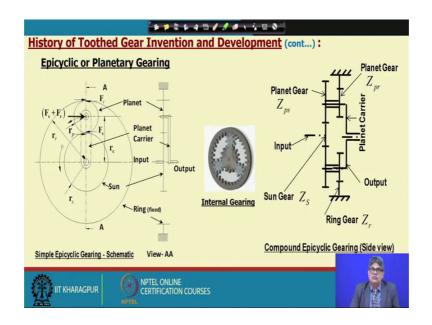
Now, internal gearing the tooth also can be generated inside the ring here if you look into here and then power can be transmitted, either the pinion can directly engaged with the internal gear or through an idler, we can have the simple gear train, we can have also compound gear train.
