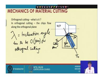
So, here first of all we see a chip coming out of the cutting zone in a particular direction and you will notice that roughly I have indicated that the chip is coming out in the orthogonal direction. What is orthogonal direction? This one, this one is the trace of the
