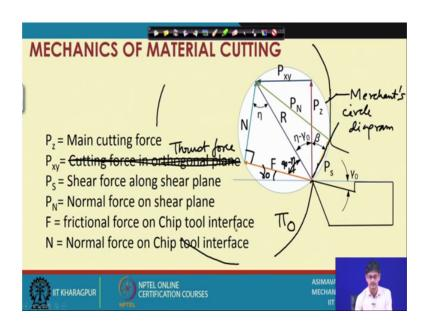
So, having agreed about that let us come to the different relationships which now exist for the resultant forces on the cutting tool. What do we mean by the resultant forces on the cutting tool? On the cutting tool the forces which are being applied by the chip they are normal force and frictional force. I mean we can break them up into such components. There is a single resultant force what we know about that force is that it is on the orthogonal plane.
