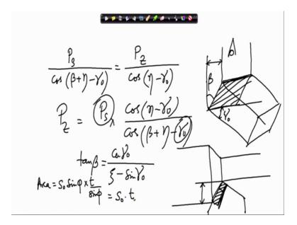
P S by cos beta plus eta minus gamma o is equal to P Z divided by cos beta sorry eta minus gamma o. From here we get an expression of P Z equal to P S into cos eta minus gamma o divided by cos beta plus eta minus gamma o.
