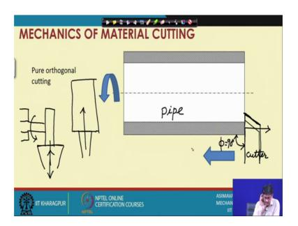
We sometimes refer to some cases as pure orthogonal cutting. What is pure orthogonal cutting? You know if we completely remove the auxiliary cutting effect, I mean the cutting contribution of the auxiliary cutting edge if it is completely removed from the picture in that case and also the other effects which are taking place if they are completely removed in that case we can have a situation in which purely orthogonal cutting is taking place with absolutely no interference from other factors.
