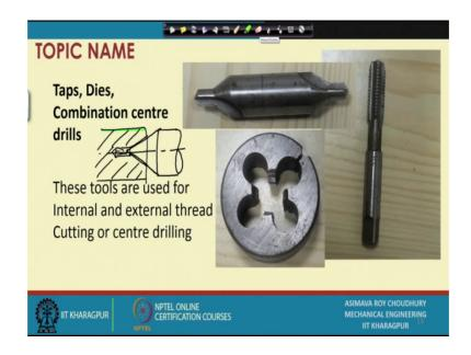
If you have a material like this, combination center drill will typically produce a hole of this type. What is the use of such a hole? Such a hole allows us to put center inside this which holds, it properly locates the axis of the body of this hole aligned with this particular center. I mean the sent the axis of this center and the axis of the body which is being held they will become aligned together.
