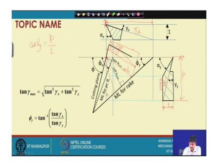
The traces of the can you see this, of the intersection of the rake surface with the base plane, now what do I mean by the base plane? By the base plane I mean that plane which is you know at the base of the tool and it is necessarily parallel to the reference plane. It might not always be parallel to the reference plane, but in this case we are ah assuming that; which is the base plane here this is the in the sectional view of the tool, in the machine longitudinal plane phi x.
