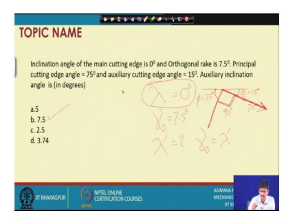
A multiple choice question, what does it say? It says inclination angle of the main cutting edge is zero degree. So, we write the information which is given here is that is right we were discussing this particular problem. So, here first of all what is given is lambda equal to 0, orthogonal rake gamma o is equal to 7.5 degrees, principle cutting edge angle is 75, this is the main cutting edge and auxiliary cutting edge is having an angle of 15 degrees.
