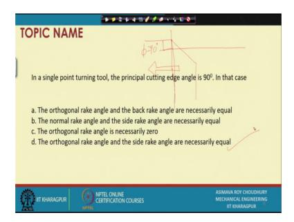
In a single point turning tool, the principle cutting edge is 90 degrees in that case. So, let us draw of a figure of a tool this is it sorry this is it a tool of this type it is moving this way and this is 90 degrees that is it.
