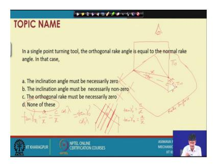
Just one moment in a single point turning tool, the orthogonal rake angle is equal to the normal rake angle in that case the inclination angle must be necessarily zero, the inclination angle must be necessarily nonzero, the orthogonal rake must be necessarily zero none of these. So, first of all let us see what is given. We are given that sorry we are given that the orthogonal rake.
