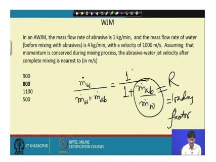
Water by m dot water plus m dot abrasive equal to if you divide this by m dot water, it becomes 1 by 1 plus m dot abrasive by m dot water and this one is called loading factor or r loading factor.
