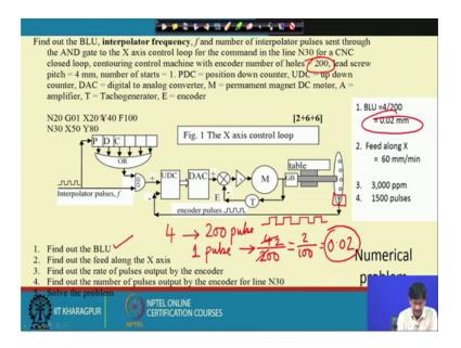
Find out the basic length unit interpolated frequency f and the number of interpolator pulse is sent through the end gate to the X axis control loop for the command line 30 for a CNC closed loop contouring controller continuous control whatever with encoder number of holes 200 lead screw pitch for millimeters number of starts equal to 1 and PDC stands for position down counter ok.
