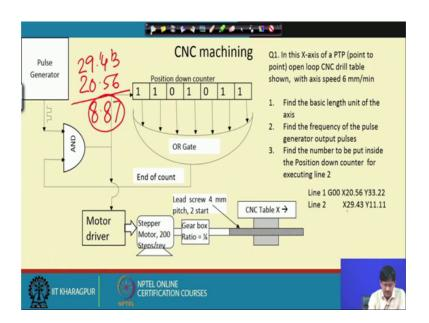
So, let us subtract it, 29.43 and it was already a 20.56; 20.56. So, this means 13, 7, 1, 14 and this is 6. So, this is 8 and 1 goes here 8; 8.87 millimeters of movement are required. So, I have to put some number. So, that this will get decremented and it will exactly become 0 when the required motion has taken place per pulse, I am having 10 microns of movement.
