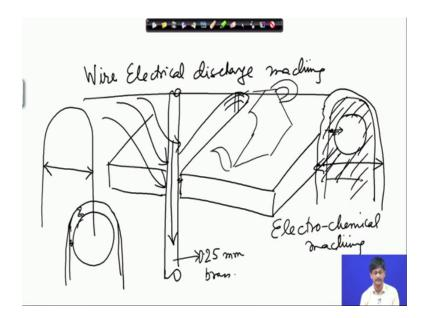
There is another method called wire EDM, wire wire electrical discharge machining which works on the same principle as you know EDM, only difference is that there is a wire which is moving and it is used as the cutting element; that means, if there is a material here say a sheet of metal and I want to cut this along this line this way I want to cut it.
