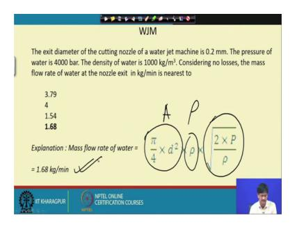
This is a sorry, this is a, this is rho and this is v how is we found out v is found out by converting the pressure energy completely to velocity energy ok.
