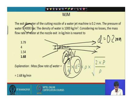
Next the exit diameter of the cutting nozzle of a water jet machine is 0.2 millimeters, the pressure of water is 4000 bars, the density of water is 1000 kg per meter cube, considering no losses, the mass flow rate of water at the nozzle exit in kg per minute is nearest to these are options and I am providing the answer 1.68 kgs per minute.
