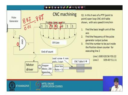
So, this means that if I want to have 8.87 millimeters of movement, how many pulses would be required? 887 pulses will be required in order to get the stepper motor move the table through 8.87 millimeters.
