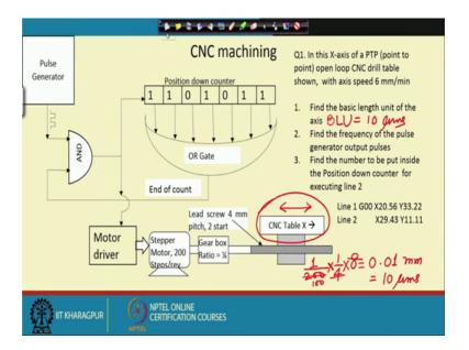
So, let us start right away with our figure that we have come across and the question reads in this X axis of a point to point open loop CNC drill table shown with axis speed of 6 millimeters per minute find the basic length unit of the axis, find the frequency of the pulse generator output pulses and find the number to be put inside the position down counter to for executing line number 2 of this particular couple of lines.
