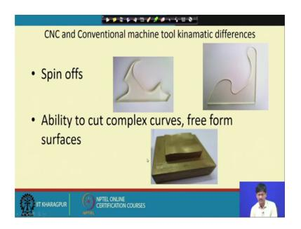
So, these are some of the parts that we have cut by computer control; see these profiles if you give this to an operator of a manually operated machine you know what we he will say; he will say this is very difficult I am going to charge you 5000 rupees in order to cut this; because I have to draw this profile very accurately on the plastic part. And then cut with great care and you have to pay me 5000 rupees with an advance of 500 rupees; now itself similar thing.
