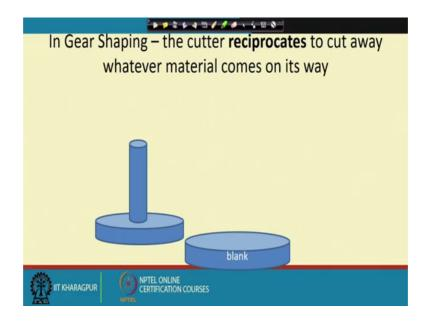
So, now we come to the idea of gear shaping gear shaping can be explained in just one sentence while 2 gears are rotating if one of them. So, if these 2 are rotating together, if one is a solid and the other is made to reciprocate this one-this one will remove all the material it meets on its way and what will result is the actual gear.
