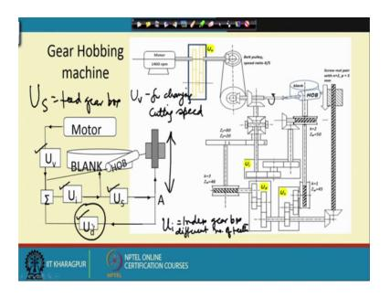
Gear Hobbing; what is gear Hobbing? Gear Hobbing means that just like a worm and worm gear they are machine ok, let me just give you the idea in simple words just like.
