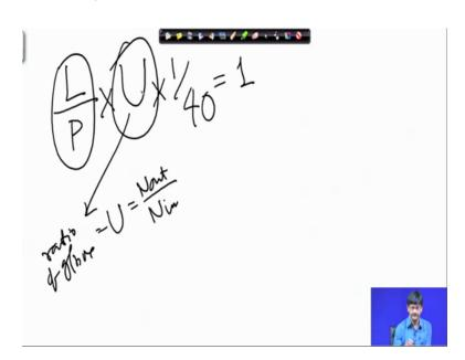
Once you get L divided by P, these many rotations enter the gearbox at the gearbox ratio is not known that is what we have to we need to find out ratio of gearbox equal to you know say U, a variable equal to actually output by n input this is the input. So, this multiplied where this will give you the n output this one multiplied by the indexing head ratio. So, it reduces the rpm by a factor of 40, this must be equal to 1 and from here we will be able to find out this value ok.
