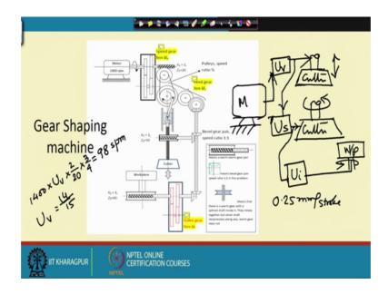
Gear shaping has a structure of this type, let us try to draw the body call it the schematic drawing, since it is not provided here. So, if we notice this is the motor this is the way you can read it this is my motor. Now what are my outputs I am first of all as we discussed the cutter is rotate a were moving up and down.
