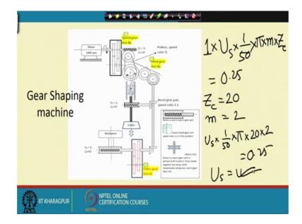
I mean rotation of one not rpm. So, U s 1 is to 1, 1 is to 1, then it enters K by Z equal to 1 by 50. This one is the number of rotations of the cutter per rotation of the cutter the cutter executes a circumferential motion of you know one circumference pi D. So, x rotations will have x into pi D amount of circumferential movement.
