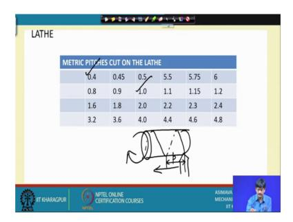
Next, now on the lead we might be having the problem that we have to cut out different threads, how do we cut threads? We have learned that we use the lead screw for cutting the threads and if we can rotate the work piece.
