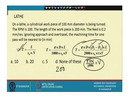
So, first of all just a moment; let me remove all the written material, so if V is given in that case we can find out N from V pi. D N by 1000 is equal to V and just by shifting terms from this side to that side numerator to denominator etcetera we can find out M.
