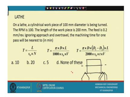
Next on the lathe, a cylindrical work piece of 100 millimetre diameter is being turned; the RPM is 100, the length of the work piece is 200 millimetres; the feed is 0.2 millimetres per revolution; ignoring approach and over travel the machining time for one pass will be nearest to in minutes 10 minutes, 20 minutes, 5 minutes none of these.
