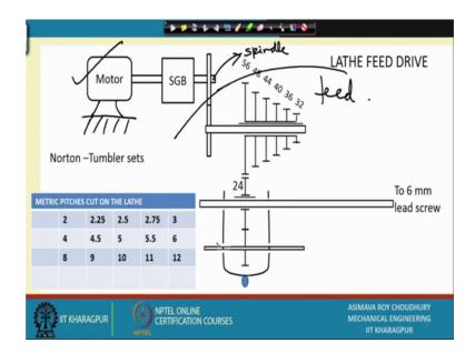
So, on the lathe we have already come across a motor; the basic motor which is providing power to the or to all the processes and in the machine; except if you are giving manual feed. But otherwise its providing all the power and we had that speed gearbox which is leading on to the spindle, which has not been shown for simplicity.
