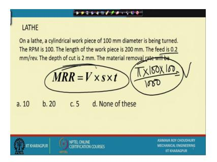
So, on a lead a cylindrical work piece of 100 millimetres diameter is being turned; the RPM is 100, the length of the work piece is 200 millimetres, the feed is 0.2 millimetres per revolution, the depth of cut is 2 millimetres; the material removal rate will be now material removal rate is given by this expression cutting velocity into feed into depth of
