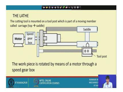
In the next slide what we see is that now the upper part of the carriage called the saddle just like we put a saddle or seat on the on the back of a horse, on top of the lathe bed seen from the top the basic body of the lathe we have put a saddle like element.
