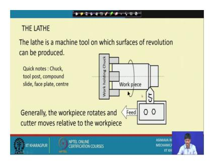
So, first of all the lathe is a machine tool on which surfaces of revolution can be produced, that is I can make a cylinder, I can make a cone, I can make a flat surface you know by which is also a surface of revolution, I can make grooves, I can make threads, I can make frustums of cones. So, all these which are surfaces of revolution I can make you know curved surfaces also, all these which are surfaces of revolution they can be produced on the lathe.
