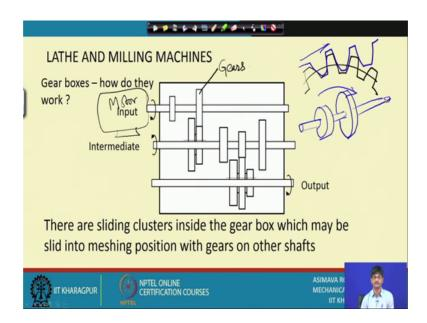
Yeah, this is the you know a more detailed figure of the gearbox that we were naming just now. What is the gearbox? You know just like we have speed gearbox and feed gear box they have some machine elements inside so that if they are you know shifted from one position to the other we would be attaining different output rotations you know output rotations of the gearbox.
