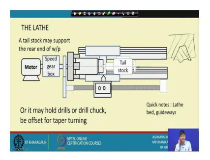
The carriage can travel from one side to the other just like a train on rails it has one straight rail on one side you know to provide enough bearing surface a flat surface is the best bearing surface and on this side in order to keep it located on a particular you know direction we have a v shaped guide. Let us let us quickly have a look at that.
