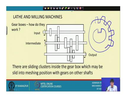
So, this is what is there on these and this sign is the sign that they are having this sort of a connection, sliding connection, key and keyway. So, let us see how the thing proceeds. So, this is the way in which it can be slid or it can come back also. You can have this position as well as that position.
