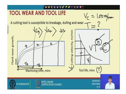
I reach the you know 0.3 millimetres at this particular time. If I use cutting velocity 2 I reach this particular limiting flank where see 0.3 millimetres at this particular time. So, this way if I use cutting velocity 3, I reach that that particular limit here.
