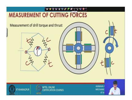
This will register a change from the null position, null position means here there is absolutely same voltage occurring here the moment they are in compression and tension this will be registering a change and from that change with calibration we can estimate how much is the drilling torque all right. So, these are some of the ways in which cutting forces can be measured.
