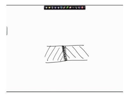
So, if I have 2 such materials this is one, this is the other and I heat them at this point, so that this part melts when it solidifies this will be a single piece. So, that we can join parts and make up shapes, our main concern is to make shapes of predetermined shape and
