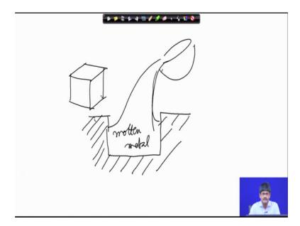
So, that we have a brief overview of the main methods of manufacturing, suppose I have a cavity, I am showing very simple principles. So, some methods some material is here. So, that a cavity is formed, inside this cavity I pour molten metal.
