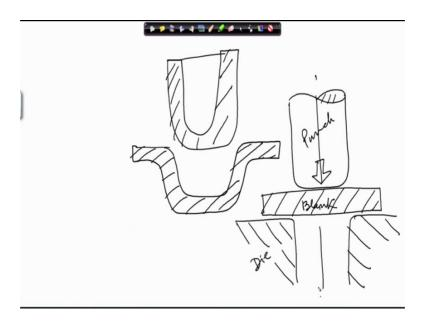
This is a very simple and explanatory example, someone shows you this part it is a sheet metal and we are seeing it only from the side a sort of sectional view, how was this done? and that particular person says that it was done by say deep drawing, what is deep drawing? So, initially there must have been a body of this type, a sheet metal piece, may be circular this way and there was a punch and there was die.
