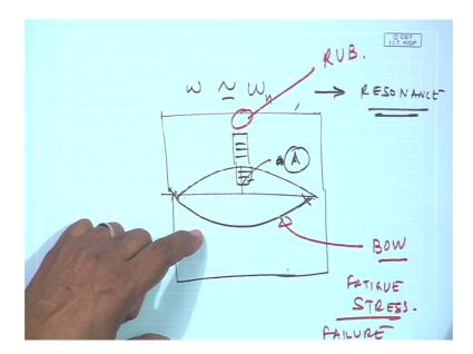
So, at resonance what happens the amplitude of the motion would increase, this amplitude could come to a level that at resonance may be this is and this amplitudes is may be undesirable or some amplitude a which is undesirable and now there are many reasons why this amplitude has to be unnerved and control.
