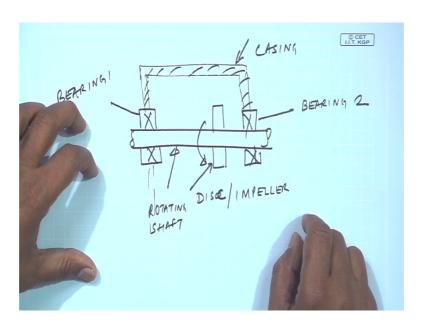
As you know every machine actually essentially comprises of a shaft which is supported on bearings and invariably it rotates and this there could be a housing etcetera and so on, if we just draw 1 half and this shaft could be carrying a disc. So, these are my bearing 2 bearing 1 this is my disc, which could be an impeller and this is the rotating shaft and this is the machine casing; I am sorry there is another 1 and this side which I am not drawing.
