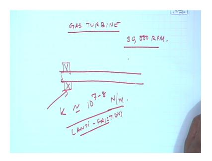
When you are operating a gas turbine we cannot really start and because gas turbines you know typically 30000 rpm. So, by the time you reach 0 to 30000 rpm when yours cranking up or start up did not start up we will cross many natural frequencies. So, you are not allowed to operate it at any of the natural frequencies otherwise residence would occur and fatigue set in.
