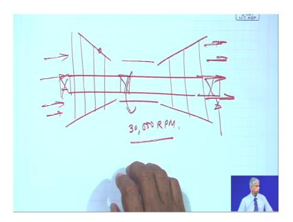
There will be sets of compressor blades you know multiple stages of compressors, when we compression chamber and then the turbine. So here going in and this shaft rotating at very high rpm 30000 rpm, so imagine if the exhaust coming out and then you get the thrust ok.
