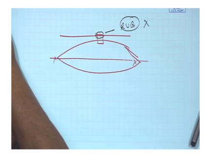
So, this is going to hit tip casing, so this rob would occur that has to be avoided and avoid torsion vibration resonance or torsion instability of the drive train system.
