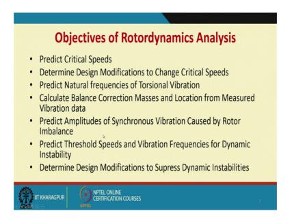
So, what are the objectives of rotordynamics, 1 is the predicting the critical speed because the shafts could be having the natural frequency because of rotation.
