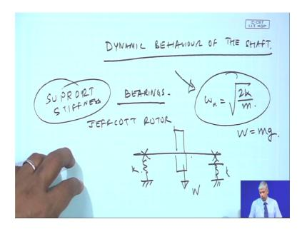
Now, what are the conditions here, it is essentially how does the dynamic behavior of this of the shaft, how does it affect the machines loosely same vibration level, let us say machine stability etcetera. Now rotordynamics we will see these bearings play a very important role and there are many simple models to study this and 1 is the simple JEFFCOTT rotor, which is nothing rotor shaft supported on bearings carrying a disc.
