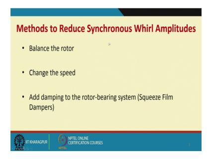
Well, to method the reduce this synchronous whirl amplitudes; obviously, if I have the balance the rotor, that means the geometric center the mass center they are all concentric and change the speed avoid the critical speed and of course add damping to the rotor bearing system in the case of the squeeze film dampers.
