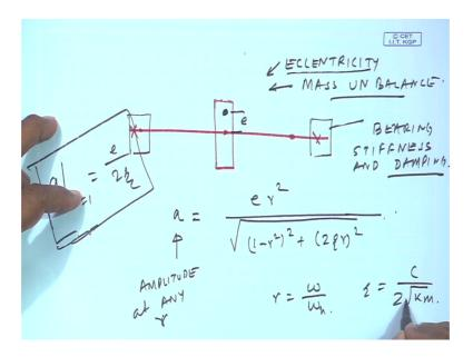
We have assumed that the shaft to be concentrated between the 2 bearings; that means, the geometry center of all the systems are in the same line, imagine if there was an or an unbalanced or an eccentricity in this soft in terms of a geometric eccentricity e.
