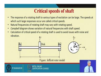
So, this is what we are talking about this critical speed, the response at such large when our critical speeds, natural frequency will vary with the rotating speed and like I told the Campbell diagram. So, the variation of natural frequencies it is shaft speeds.
