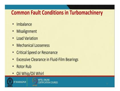
So, some of the common fault conditions in turbo machinery which we will be seeing later on is imbalance, misalignment load variation, mechanical looseness, critical speed or resonance excessive clearance and fluid film bearings rotor rub oil whirl and oil whipping.
