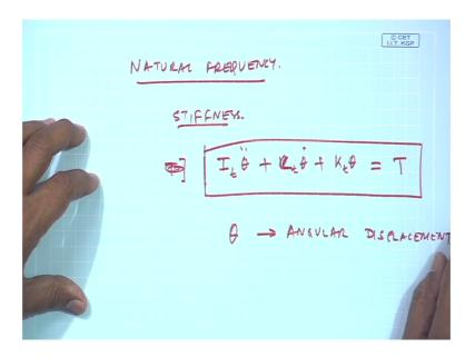
So, 1 should always avoid operating the shaft at the critical speeds, we can do certain design modifications to change critical speeds; so playing around with the stiffness predicting the natural frequencies of torsional vibration. So, far we had studied about the linear vibration, but in the torsion vibration systems I have what is known as the inertia
