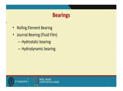
So, this bearing plays a very important role in the shaft. So, we have this rolling element bearing and the journal bearing or the fluid film bearing. So, in the rolling element bearing as I was telling you they have almost a constant high stiffness, but in the hydrostatic bearing or the hydrodynamic bearing, we can play around with the bearing stiffness depending on the viscosity of the oil depending on the eccentricity and so on.
