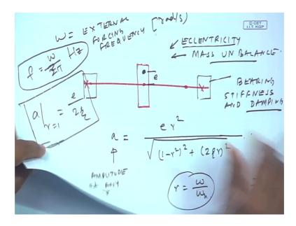
Omega n is the natural frequency system and omega is the external forcing frequency of causes this is circular frequency. So, the unit is radians per second and not hertz, where f is equal to omega by 2 pi and this given in hertz.
