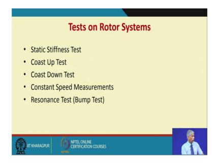
So, certain tests are done on the rotor systems, 1 to find out the natural frequencies 1 is the static test stiffness test.
