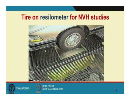
So, to understand the vibrations being produced in a vehicle; this was work which I was doing during my postdoctoral fellowship. And these understand the role vibrations coming into the vehicle, so one can work on the transfer path analysis.
