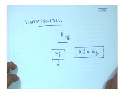
So, if you go to the market today you will find many such isolators; no this vibration isolators, which will come with an K effective, but this spring or the isolators must also withstand the static weight of the body say m g is a force. So, they should be able to withstand the static force K delta should be equal to m g. So, I can find out whether I require you know 5 numbers of spring or 6 numbers of spring and that is what is required when we design isolators.
