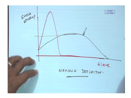
So, this is my shock energy; very high peak they will arrest this, but they will do it like this; same energy they will dissipate within less vibration amplitude. So, this is the function of shock isolators, so limit of such short isolators is the maximum deflection.
