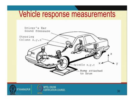
And then this is the steering wheel; suppose one does not understand; light the vibration, we can who as a vehicle designer; we have to play with K and C and either this could be done in the proving ground or this can be done in the laboratory, where there are roles on to which we can put different tire patches and this is what is actually done.
