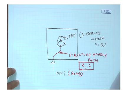
So, transfer path analysis; I have some input, I have some output. Output may be could be a steering wheel vibration because there is always a path; structure one path for the vibration energy to come from the road input to the steering wheel variation. So, in this structure one path; I can play with the stiffness and damping K and C.
