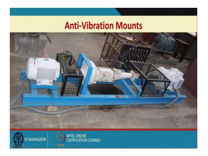
Now, this is you see these are all mounts; vibration mounts if you can see. This is the motor, it is a gearbox or the generator and so on. If there is any vibration in this frame, I
