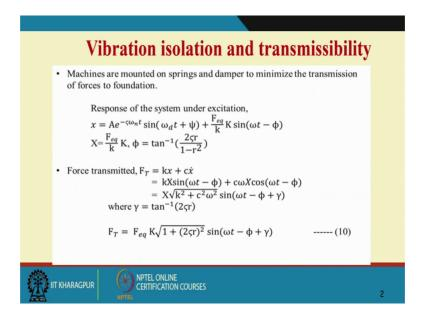
And this helps actually in the design of foundations of machines. So, machines are mounted on springs and dampers, as you know by now to minimize the transmission of forces to the foundation.
