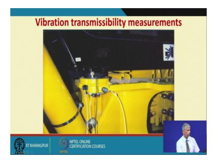
And this is how the vibration transmissibility is been measured, we will see transducers measuring on the frame and transducers measuring on the cabin of the cab and this is supported by isolators.
