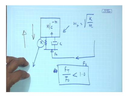
So, if I have a machine; it has certain mass M. So, if I have an applied force F naught coming into this ground. If I do not want anything to get transmitted into this body because it is a sensitive body, I can play around with this omega n of this body; omega n is nothing, but root over K by M. So, I can play around the stiffness of this bodies foundation, as to not allow this transmitted force F T should be less than 1.0.
