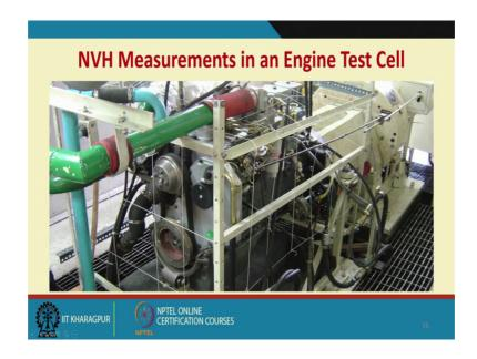
And this is a measurement being done in the engine test cell, which is again isolated because I do not want external vibrations to come and disturb my measurements.
