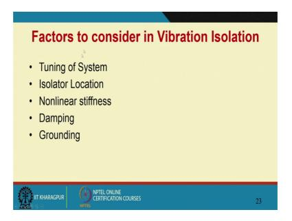
So, this will help us put where the transducers need to be put. So, factors to consider in vibration isolation; tuning of the system, isolator location, non-linear stiffness, damping, grounding has to be taken into account.
