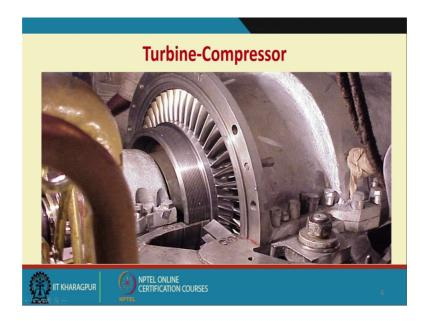
And this is the view of the turbine compressors; I am just show you this right now; so that you know what we are getting into when we talk about condition monitoring of a gas turbine. So, this will give an example to see the magnitude of the problem. You see this, such fine clearances between the outer shell and the rotor and these are all the blades which rotate at high speeds and are subjected to high temperatures.
