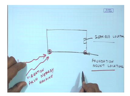
Many a times the transducers where when we measure will be at the foundation mount locations or the bearing locations but as a sterling you; the vibration from a nearby machine will always influence your measurements for a particular location. So, one has to very careful as to understand that this machine has been having proper foundations and what are the limits of the oscillators.
