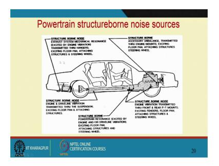
So, if you see in an automobile to reduce the structured warmth; they have a lot of isolations being put in all these locations to reduce the noise being reduced, if generated because of the vibrations of the power trim in the drive line.
