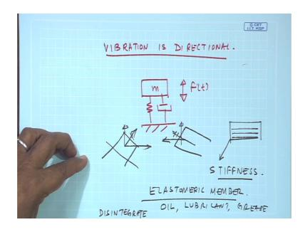
So, one has to keep in mind the predominant direction; imagine I have a body like a prush; forging prush, so all the forces are along this direction. So, I need to put isolator in this directions but many a times this is and if you will see here; isolators are put on a plane of 45 degrees; so, they will give some component in this direction also.
