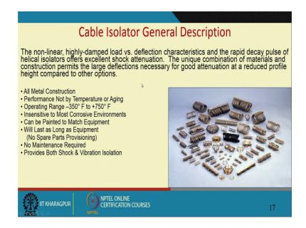
So, there are many different forms of cable isolators; they are all in metal, construction, they will not affect because of temperature, insensitive to corrosive environment and that
