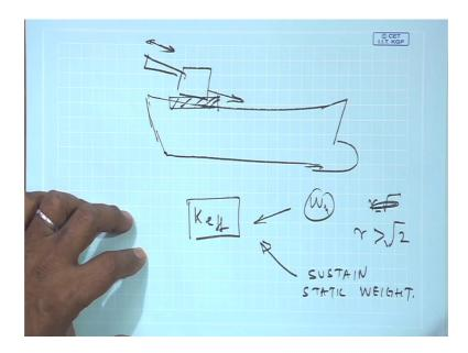
Imagine in a ship, you have a large field gun imagine you fire this gun and then there is big amount of recoil. If this recoil was not arrested, but such observers; vibration observers what would happen to the motion of the ship? A lot of fatigue in these stresses would occur. So, this is arrested by this heavy duty cable mount isolators.
