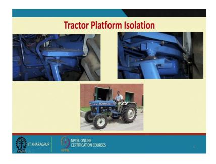
This is one example where in a tractor see the foot pedal; the driver puts his foot on this platform and this underbody is rigidly connected to the engine of do the frame of the track. So, all the unbalanced forces which occur in the engine during combustion is going to excite the structure and there will be a large amount of provisions. So, I do not want this platform to vibrate, so the transmitted force has to be less.
