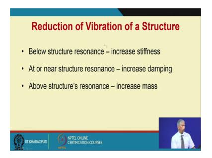
So, reduction of vibration of a structure; act resonance, increase damping, below structural resonance, increased stiffness and above structures resonance increase mass.
