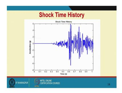
But once I have talked about vibration isolation, I must tell you about shock; many a times shocks are very very high frequency impulses for a very very short duration.
