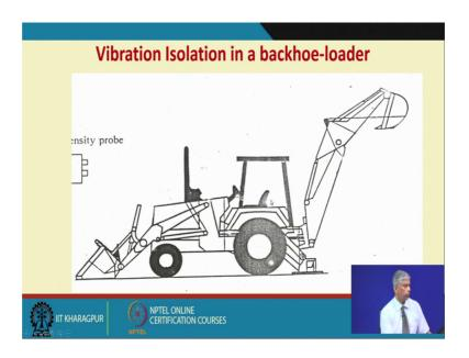
So, you will see an example where in a backhoe loader because this cabin beam is put rigidly on the frame of the backhoe loader. And this backhoe loader is subjected to large amount of forces because it is doing off highway operations, so this driver seat has to be isolated.
