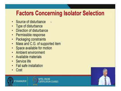
Well, one has to be very careful about how to put these isolators. So, we need to know these sources of disturbance and in particular the center of gravity of the supported item.
