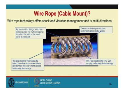
As opposed to wire rope or cable mounting; cable mount it is multi directional that is the advantage of such cable mounts. The reason I am showing you this is when you go to the industry, you will see many such applications of isolators; be it cable mount or be it helical spring. Now this kind of isolators are there and then we have to measure at these locations when they are mounted to these machines.
