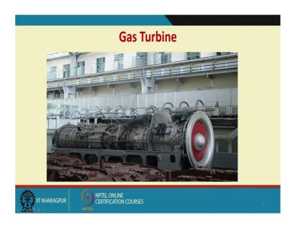
Same is to for gas turbines; gas turbines are put on a bay wherein they are rotating at very very high speeds. Imagine a small amount of unbalance because the speed is so high there will be lot of forces coming onto the frame. So, they have to be of course, you know in gas turbines we perfectly balance it. Nevertheless there has to be good oscillators kept everywhere.
