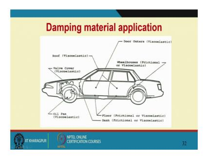
And then we can put damping materials to reduce the vibrations.
