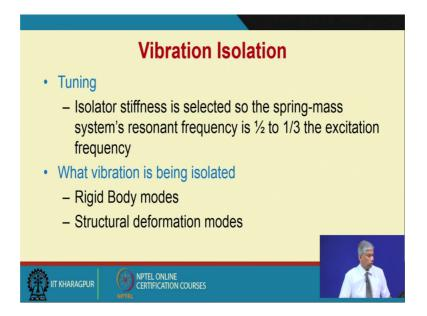
So, all if you must remember that vibration isolation; we need to find out the natural frequency and the frequency response should be less than or greater than root 2 so that the force transmitted force is less than the applied force.
