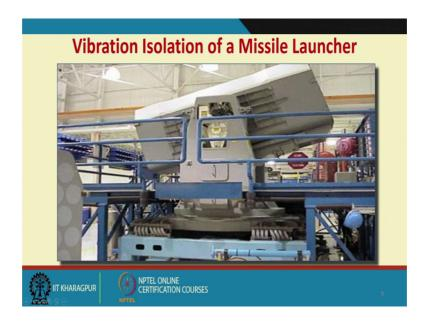
And you see this one another missile launcher; wherein we have cable mounts being put so that the recoil is arrested and then large motion is not being propagated.
