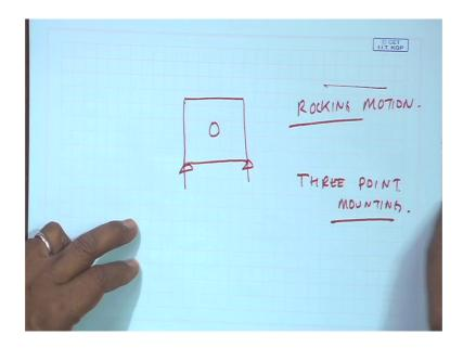
So, otherwise; this is not geometrically balanced; there will be always supports are not geometrically balanced we will have a rocking motion.
