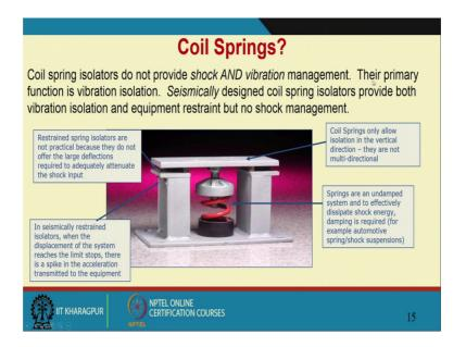
So, in many applications you will see shocks needs to be isolated. So, vibration isolators are actually done by coil springs, so coil springs isolators does not provide; they provide primarily vibration isolations; all if you can read this.
