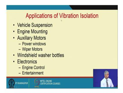
So, vibration isolation is there in a vehicle in almost everywhere; vehicle suspension, I showed you the example of that wavy road, engine mounting many auxillary motors like the power windows, wiper motors, windshield washer bottles, the electronics. So, all of these will get affected if they are not properly isolated.
