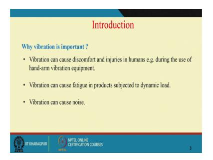
So, why vibration is important, (Refer Time: 07:22) vibration can cause discomfort injuries in humans during the use of hand arm vibration equipment. You must have seen in the people holding jack hammering equipment in order to break concrete etcetera, at their hands they will be exposed to high levels of vibrations and they may have
