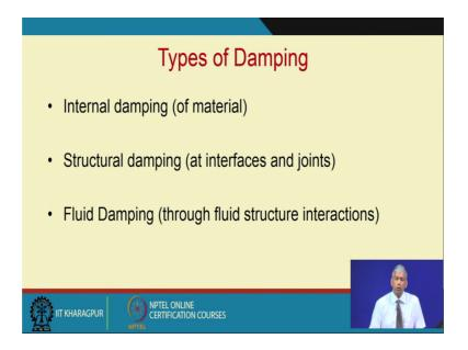
And many a times in materials this is all internal damping, structural damping at interfaces and joints, and fluid damping through fluid structures and interactions. So, this dampings control the response and we must have a good idea of estimation of the dampings in the system.
