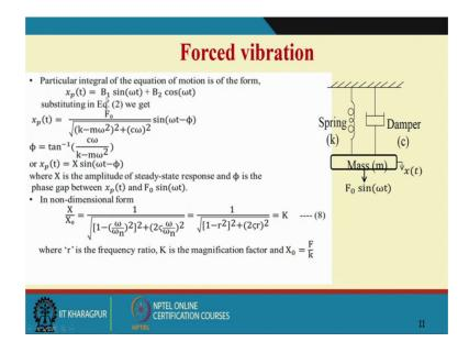
We will continue the discussion to the force vibration for the particular integral solution. So, I can have a response like this you want sin omega t plus B 2 cosine omega t. If I substitute this I will have the particular integral in this form given by a phase, phase is
