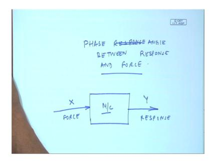
So, many systems we need to find out the natural frequency of systems. So, looking at the phase response between or phase angle between response and phase and force we can find out the natural frequency.
