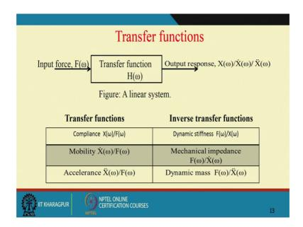
Now, we have seen this was for a single system, but many systems you will see that there is an input and there is an output this could have been force and this could have been response and this could have been my machine or a system excuse me.
