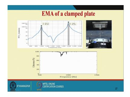
So in fact, if you look at the system this system has many degrees of freedom and right now we have just shown you the two natural frequencies of a clamp plate and there is a coherence which I will describe you later on as the causality between the input and the output. And this means the force is only producing the response and so on at almost all the frequencies.
