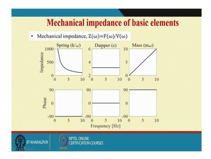
So, this is like an homework for all of you to find out the impedances of few mechanical systems like a spring damper and mass and I just show you what this impedance value is. So, you can given force, harmonic force find out the displacement, find out the velocity and find out take the ratio to find out the impedance.
