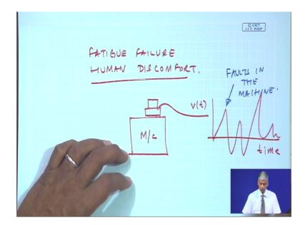
But in machinery condition monitoring we have a transducer on a machine and we get this vibration signal v t something like this. So, it is by analyzing this signal which we will discussed the techniques of analysis later on we can find out what is the faults in the machine.
