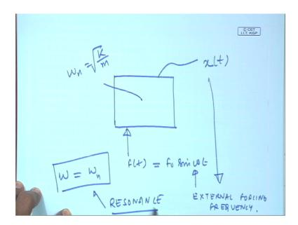
So, we will see this response will actually be at a frequency equal to omega, but this body has certain stiffness and mass, so it has a natural frequency. When the external frequency omega is equal to omega n we will have a condition of resonance and this has to be avoided at all.
