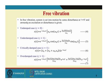
So, in the free vibration case at t is equal to 0 we will give there is no excitation or disturbance and there will be few cases when we have zeta equal to 0 undamped case because damping does not exist. So, this could be one solution and then underdamped case critically damped and overdamped case. We will see the plot of these responses of this body to this kind of damping scenarios.
