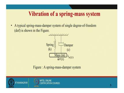
Now, let me take the case of a single degree of freedom system where this is a body rigid body of mass m it is only allowed to move in this x direction as shown here. So, basically though if it was in space it could have moved in 6 degrees of freedom. But I am
