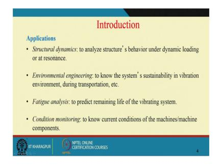
So, lot of application of these vibrations in structural dynamics to understand the dynamic loading at resonance, to know the systems sustainability in vibration environment, fatigue analysis and of course, lastly which is important for us is know the condition of the machine components because of the vibration it is producing.
