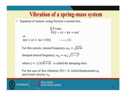
So, I have mx double dot plus cx dot plus kx is equal to F t is the equation of this motion now there can be many solutions to this equation differential equation and this is the first order linear differential equation.
