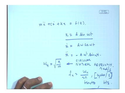
So, x is equal to A sin omega t can be a solution to expression and if I substitute x dot is equal to A omega cosine omega t and x double dot is equal to minus A omega sin omega t, in the above equation I will come up with an expression where omega n is equal to root over k by m and which is known as the natural frequency of the system. It is a circle on
