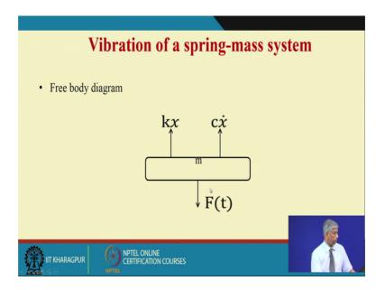
So, if we look at the free body diagram of this body there is a resultant force and then there is of course, the body it has not been shown because it has been balanced by the static deflection. So, the net force will be shown this way wherein the net acceleration of the body is given by this expression where f is the external force ok.
