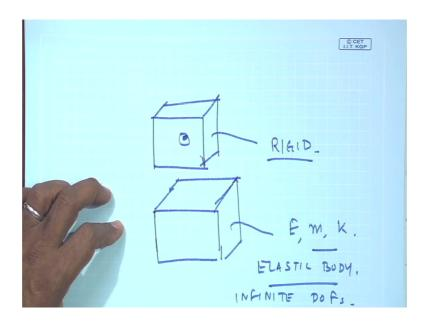
So, in elastic body or body which will deform they will have infinite degrees of freedom for the sake of understanding we will be right now considering the rigid body vibration of a body of mass m about its center of mass.
