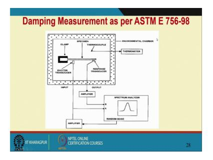
And this is an experiment in the lab wherein we are exciting and we have in response to find out the damping in a cantilever beam.
