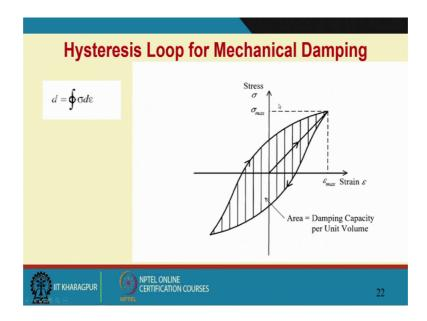
The statically loop because of mechanical damping. So, metallurgists are developing materials with high damping capacity so that the vibrations could be reduced like the cylinder block of an engine having materials, having high damping and so on.
