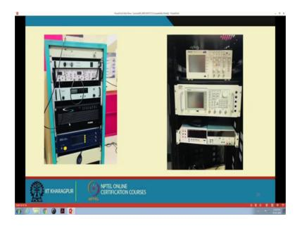
My students do a lot of signal processing algorithm development with this an industrial PC. The signal analyzer for the laser parameters, this is an amplifier for the electromagnetic exciter, this is a filter wherein you can have a low pass high pass or a bandpass setting.
