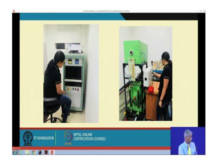
This is the control panel of that same engine where the student and of course, this engine is connected to an eddy current dynamometer where all the load tests can be done, the efficiency calculations going to be done and then you can see this motion test where one of the engine cylinders is being misfired.
