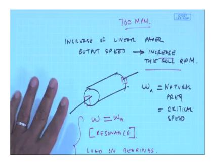
So, increase of speed, increase of linear paper output speed would mean increase the roll RPM. But you know by now when I have a roll or a shaft it has certain rotational natural frequency or what is known as its critical speed. So, by increasing the speed I may so happen this increased speed may become equal to omega n. So, I will have the condition of resonance. So, resonance means large motion. So, this will be long stable and then eventually things may fail or break that is one.
