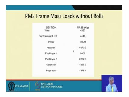
And of course, to do such analysis we had to take the mass of these units, and on this you can come get from the cad models and once you have the density we can get the cad model from the cad models mass can be estimated.
