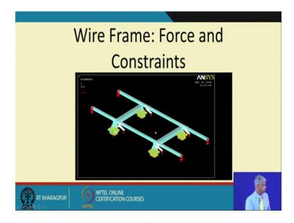
The major components are modeled once the cad was available we needed to have the FEM model showing the locations of the forces and the constraints.
