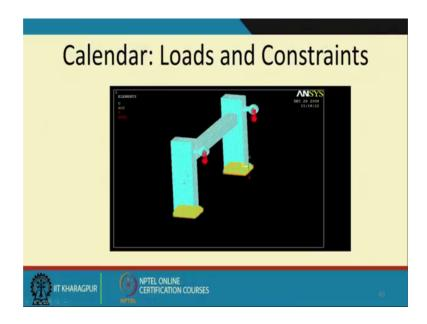
So, all the frames of the paper mill, all frames supporting the rolls stress analysis is to be done and also modal analysis.
