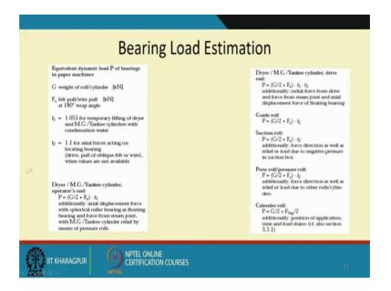
So, by the way to estimate the bearing load estimations this is the weight of the roll of the cylinder and then the angle of wrap needs to be known. So, you can calculate the dryer or the M G roll, these are the rolls you can calculate the loads similarly for the dryer summer for the guide roll, suction roll, press roll, calendar roll. So, all these expressions are known to estimate the loads.
