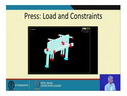
Similarly, for the press, loads and constraints are given the because these are all the frames. So, if these hold the rolls the forces come onto these frames and then we can estimate the loads.
