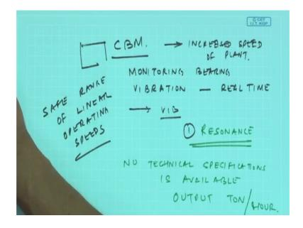
But if then somebody increase the speed of the plant, these vibrations would increase and one has to be safeguard against resonance.
