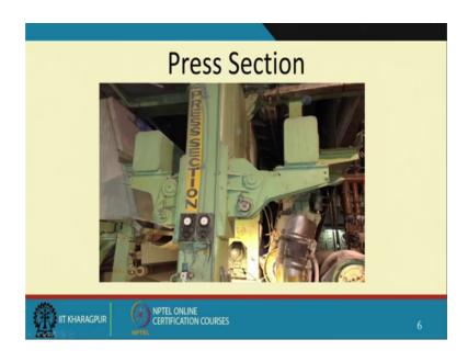
And this is in the pressing sections you can see a big roll here ok. So, they are hydraulically operated ok.
