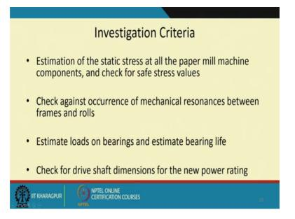
So, our investigation criteria was estimation of the static stress at all the paper mill machine components and check for safe stress values if they were not safe we need to reinforce structurally. But mostly is important is check against occurrence of mechanical resonances between frames and rolls because the frame has a natural frequency the roll
