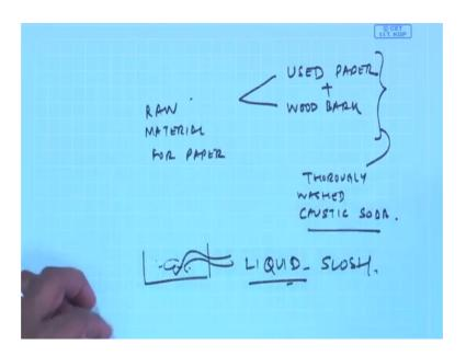
So, when we the raw material for the paper is actually either used paper or wood bark or a combination of them and they are thoroughly washed with caustic soda ok, and this forms a very liquid slosh is there. So, when such slosh is fed onto the wires I will show the pictures in a little bit and then basically if they are pressed the initial pressing is the water the squeezed out and this will be a wet damp layer of paper which would come out.
