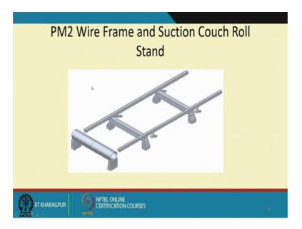
Now, this is an CAD modal of the wireframe and suction cultural stand this is right in the beginning. So, this is the suction coat stand and in the wireframe ok.
