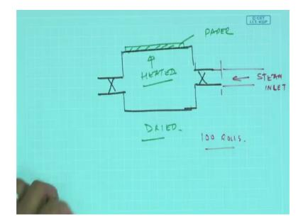
Each of the dryer rolls is supported on bearings, but then they are connected to stream inlet. So, the paper which goes in here is heated and thus it is dried. So, one roll is not sufficient enough to give the amount of heat required. So, they have to be continuously. So, these dry rolls there could be 100 such rolls in standard paper mill ok.
