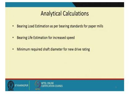
So, and then of course, the analytical calculations was bearing load estimation as for the bearing standards for paper mills, bearing life estimation for increased speed, minimum required shaft diameter for new drive reading. So, this was done.
