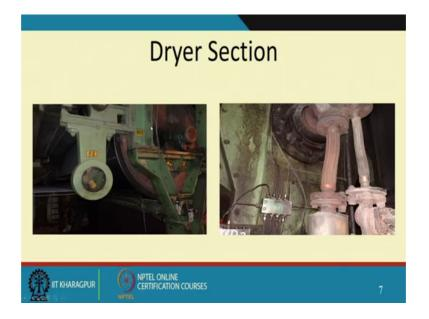
Then this is the view of the dryer ok, you can see a big dryer which are streamed right and this is a big roll driven by an individual motor sometimes, sometimes and then this is the bellows through which hot steam is inserted inside the drum the dryer rolls are actually hollow drums.
