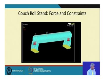
Similarly, for the couch roll force and constraints these are the constraints because they are the bonded the yellow colors and the red one are the forces coming at the bearing locations.
