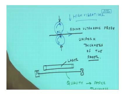
The paper comes out and it is actually pressed. So, we have a uniform thickness of the paper. In fact, to measure the thickness there is a roving ultra sonic probe along the length and breadth. So, this is a paper supported and rolls there is a roving ultrasonic paper and sometimes it is an ultrasonic or a laser beam is used to measure the paper thickness.
