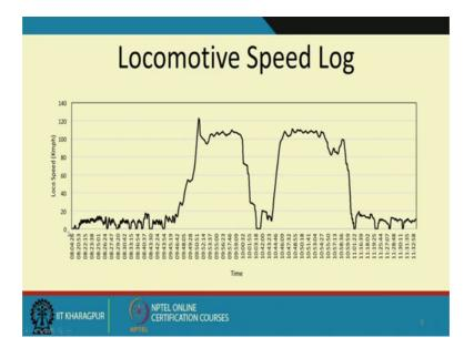
And you see this is the local speed in kilometers per hour and this we pulled out of the data logger and this is the actual time, we started somewhere from Kharagpur around 8 in the morning.
