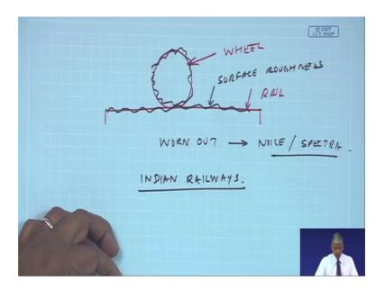
So, if tracks get worn out, they will produce a noise of a different spectrum.
