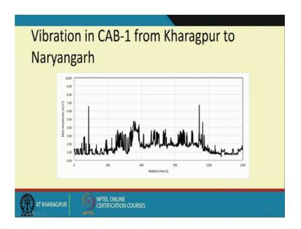
And then if you look at the vibration level from 0 to 10 meters per second square. So, when the you are running comfortably these levels are on the floor of the cab about, 2 to 3 meters per second square ok.
