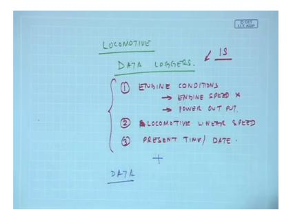
Now, also have data loggers wherein as soon as I start the engine it will keep a log of the engine conditions by mean what is the engine speed and the power output ok. The reason this power output is very easily measured and because these diesel locomotives actually have an electric serious traction motor.
