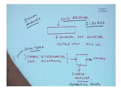
This data recorder is an 8 channel that recorder, which takes only voltage input the max of 10 volts. But when we have the accelerometer or the microphones they will give you a voltage amplifier voltage signal only if they have been conditioned with their corresponding charge amplifier.
