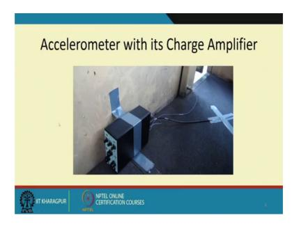
Now, this is a view of the charge amplifier used for the accelerometer and you can see how this duct tapes come handy to anchor it there are temporary anchoring, because I do not want to; obviously, permanently mount these and then you can see the accelerometer mounted in the door column of the cab and these cables are always strapped down.
