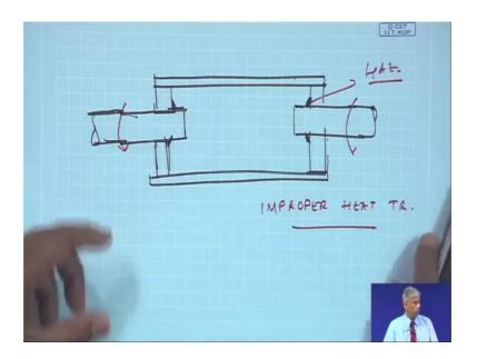
How go these are again welded. So, there are a lot of failure in this realm and areas and this on top of it this belt goes over it and these are made to rotate ok. So, HAZ and improper heat treatment it was the reason and this was discovered by doing a chemical analysis of the component failed component and again.
