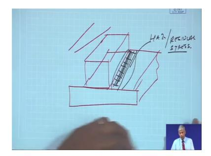
So, again when we weld a structure so, if you put a well band here so, some of the zones they will be heat affected because at the high temperature ok. So, there will be residual stress build up and then on top of it, if it is subjected to residual fatigue loading they will be quick freely, I have seen in my book you can see a filler analysis of a band pulley in a conveyor system.
