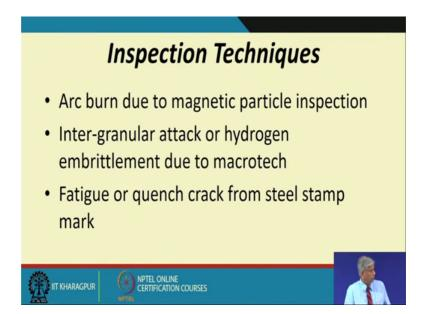
Some of the inspection techniques are burned due to magnetic particle inspection intervener attack or hydrogen embrittlement due to macro tech fatigue or quench cracks from steel stamp mark. So, all this would lead ok.
