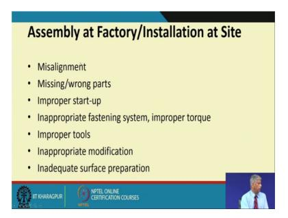
Again failures can occur because of assembly at factory installs inside misalignment, missing wrong parts, improper startup, improper inappropriate fasting system, improper
