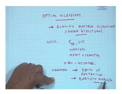
Any extra heat which has been generated when preparing the sample is going to damage this component ok. And then all the mechanical properties whatever we can measure like yield point or ultimate or hardness impact strength ok, but since the sample is very very small we need to have known nowadays you know we have nano indenters wherein we can find the hardness as a function of depth of penetration.
