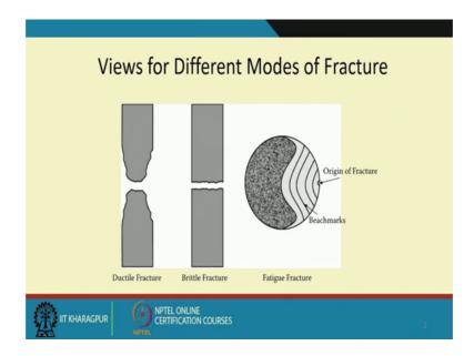
So, well materials will fail materials will fail because and looking at the failure we can know what is predominant the reason of filling a ductile material if you fail it would make a cup and cone like a form. So, looking at the failed component and those of you who are students you would have seen, when you do a uniaxial test of mild steel specimen in an UTM Universal Testing Machine.
