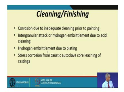
In many of the cleaning finishing operations corrosion due to inadequate cleaning prior to painting, integral under attack or hydrogen embrittlement due to acid cleaning.
