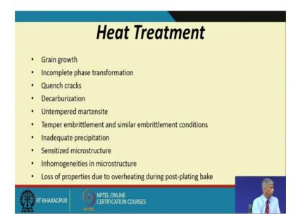
Similarly during heat treatment, you know the time TT time temperature ok. How quickly we bring down the temperature as a function of time helps developing micro structures, where a whether martensite is formed per lattice form it all depends on the cooling rate ok.
