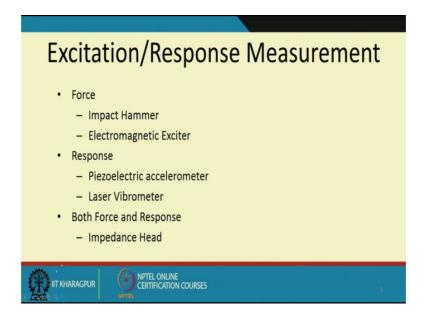
So, in summary; to give forces to a system I can whether I can either have an impact hammer or an electromagnetic exciter.
