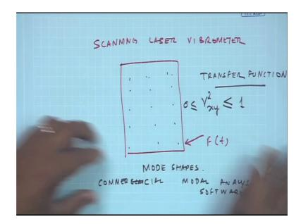
There are scanning laser vibrometers available. So, in one go suppose I have a panel and I am exciting it by some force F t. So, in one go it will measure the responses at all locations with the right phase reference keeping one as a phase reference and then you can get a entire picture of how this surface is vibrating.
