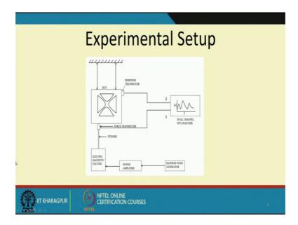
Sometimes through similar trail conditions we can hang them by strings, they are simply supported or they can be put on air cushions etcetera. So, this is my response transducer and this is the random noise generator instead of random noise generator; I could have a sine sweep, I could have a sine signal I could have a chart signal.
