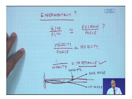
But question is how do we find experimentally these conditions? As you would have seen this response x double dot by F both in the frequency domain this is nothing, but a ratio of the response to the force to the force.
