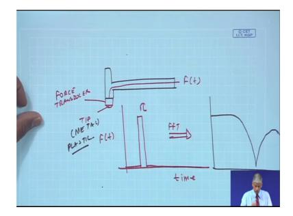
So, this hammer actually nothing but looks like in hammer and here on the tip we put a force transducer and there could be a some tip material and of course, we have the cables to give you a signal F t.
