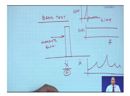
And you must have heard what is known as a bang test bang test is you know we just excite the structure with a blow; a hammer blow. Basically this means what? It is giving an impulse and in the frequency domain an impulse would look like a flat response. So, if I am measuring X by F and if this happens to be a constant.
