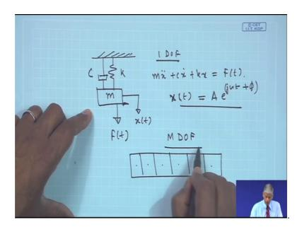
So, we have to determine natural frequencies, modal damping, mode shapes. Now if you consider a dynamical system for example, a mass spring dashpot or damped oscillator.
