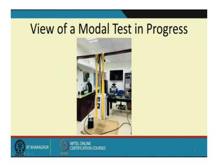
And this is just to give you an example of we are doing the model testing in our lab of a portable air conditioner. And if you will see here there is an dual channel FFT analyzer; this FFT analyzer has a signal generator which is feeding this power amplifier here.
