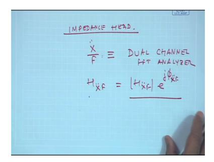
So, such transducers are used which can measure both acceleration and force at the same time and these are known as impedance head ok. So, we require either an impedance set or separately a force transducer and an accelerometer.
