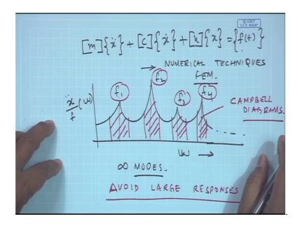
Now as you would have seen in the techniques of Telamon method I can modal this body as a system given by this matrices. Through numerical techniques I can find out the responses of this body like FEM etcetera and then find out the natural frequency. So if I have a multi degree freedom system and if I look at the response x double dot by the force maybe in the frequency domain.
