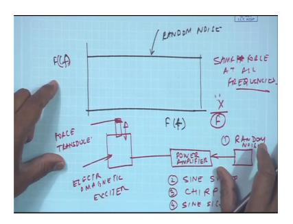
Another method of excitation is this electromagnetic exciter wherein I give a random noise and this is generating a flat frequency to a large extent. So, there are commercially available electromagnetic exciters which will be having a power amplifier to which I can give a random noise.
